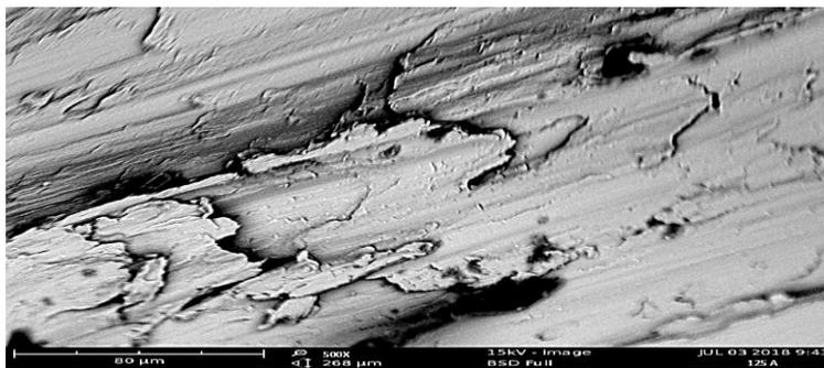
**Plate 4. Fracture Surface of Test Specimen of High Heat Inputs at 500X Magnifications**
