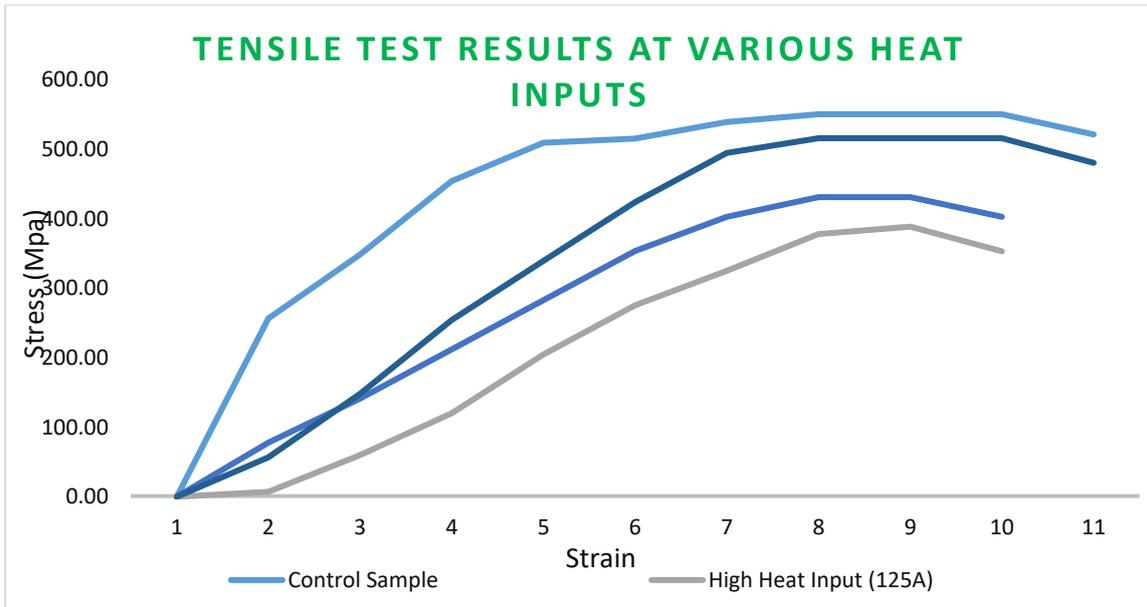
**Figure 2. Tensile Test Results of the Samples**
