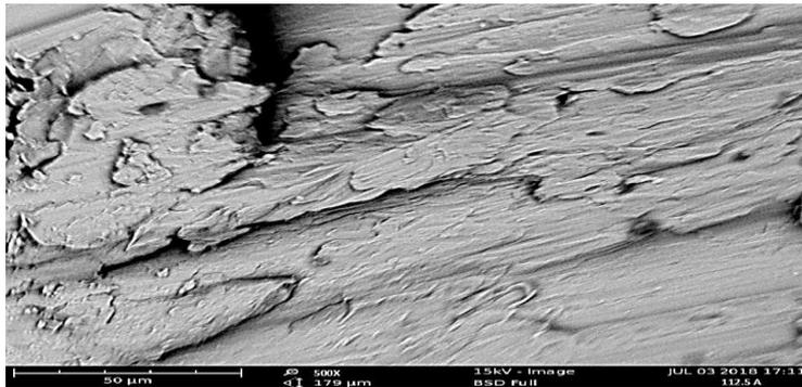
**Plate 3. Fracture Surface of Test Specimen of Medium Heat Inputs at 500X Magnifications**
