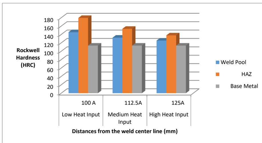
**Figure 1. Micro-hardness results at different zones of the weldments with different heat inputs.**
