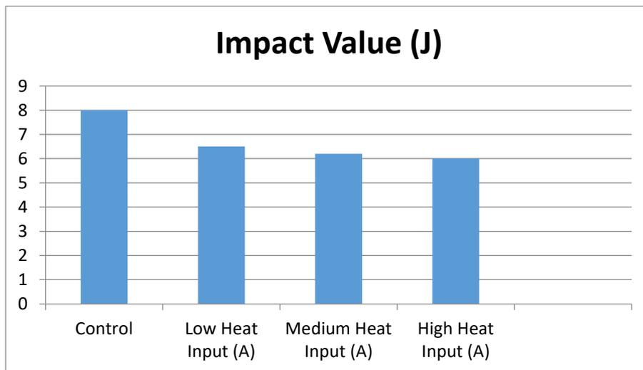
**Figure 3. Impact Test Results at Different Heat Inputs**
