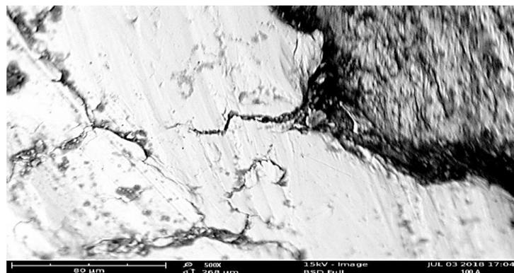
**Plate 2. Fracture Surface of the Test Specimen of Low Heat Input at 500X Magnifications**
