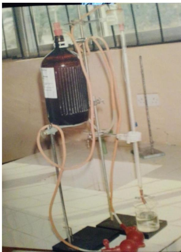
**Figure 6:** *The photograph of the designed positive pressure dispenser*
