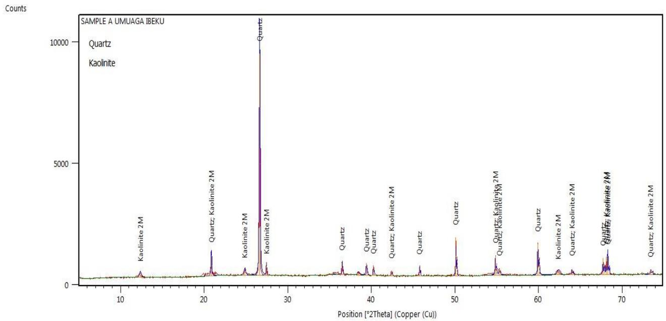
**Fig. 12** Mineralogical X-Ray Diffractograph of Umuagu Erosion Site Eroded Soil
