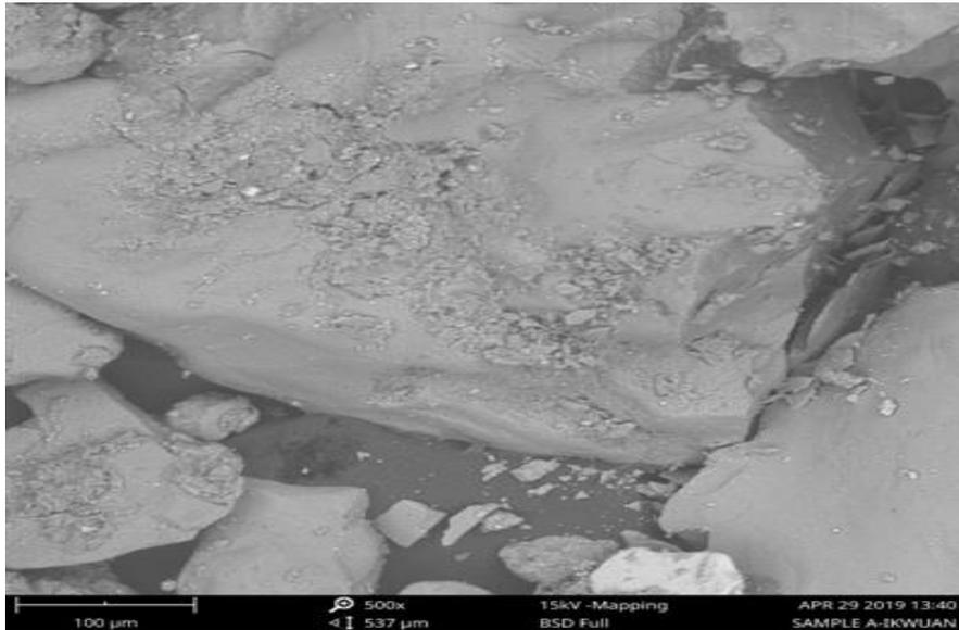
Fig. 8 Scanning Electron Microscopy (SEM) morphology of Ikwuano eroded soil 100μm and 500x exposure
