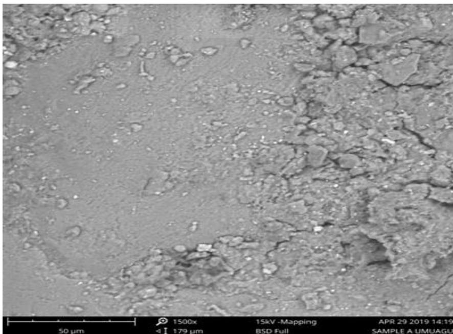
Fig. 7 Scanning Electron Microscopy (SEM) morphology of Umuagu eroded Soil 50μm and 1500x exposure
