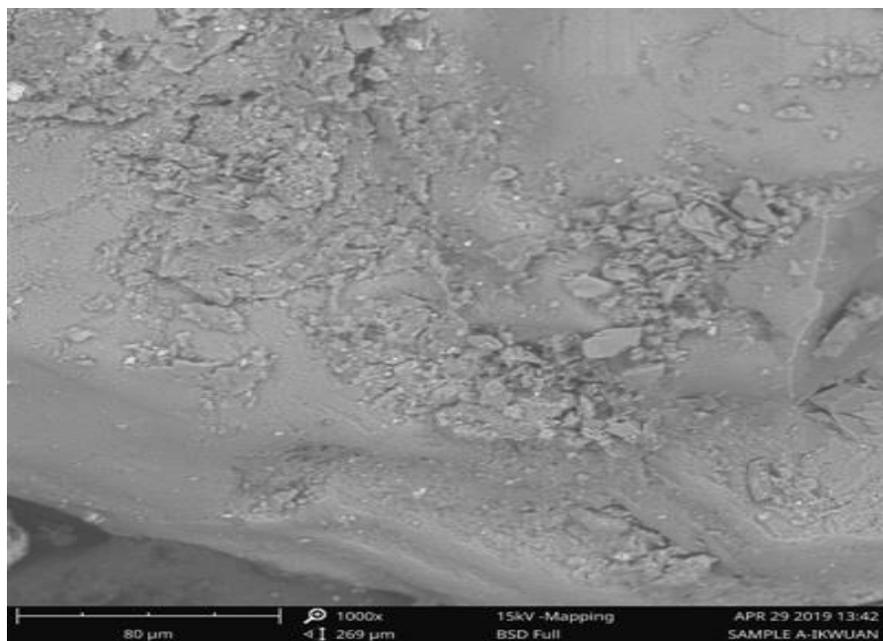
Fig. 9 Scanning Electron Microscopy (SEM) morphology of Ikwuano eroded soil 80μm and 1000x exposure
