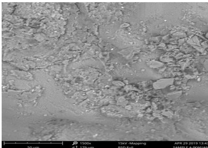
Fig. 10 Scanning Electron Microscopy (SEM) morphology of Ikwuano eroded soil 50 $\mu$ m and 1500x exposure
