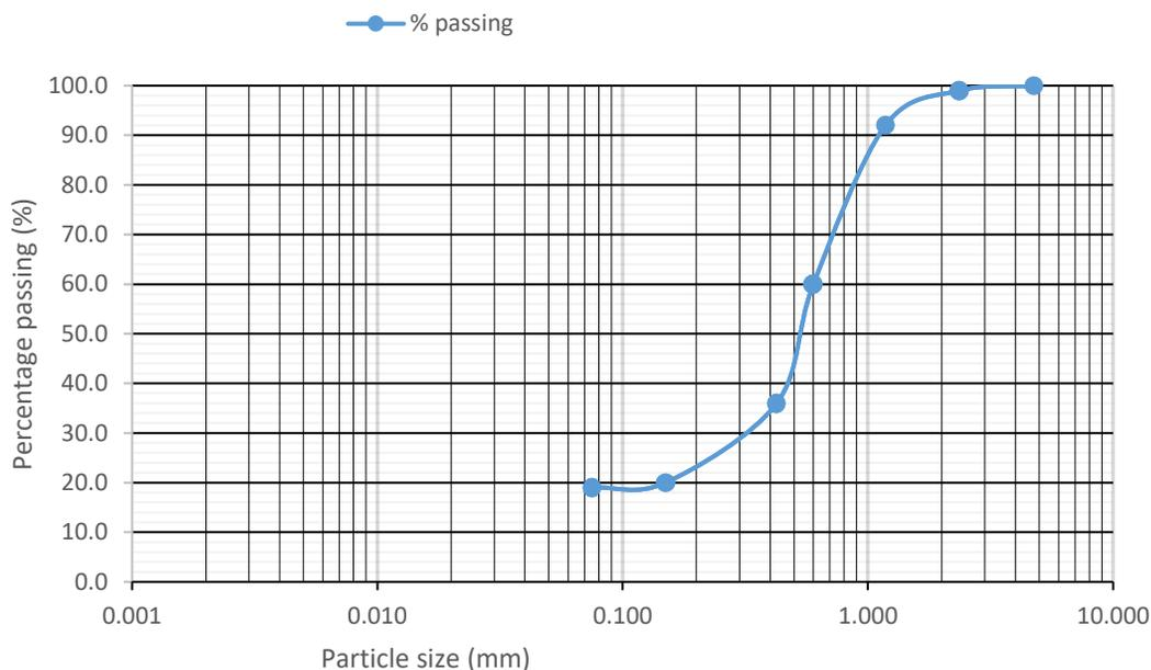
Fig. 2 Particle size distribution of Ikwuano studied eroded soil
