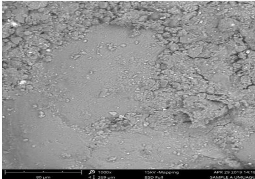
Fig. 6 Scanning Electron Microscopy (SEM) morphology of Umuagu eroded Soil 80μm and 1000x exposure
