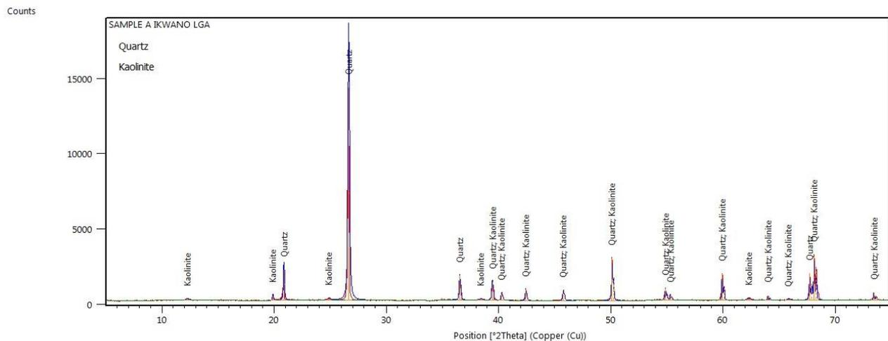
**Fig. 14** Mineralogical X-Ray Diffractograph of Umuagu Erosion Site Eroded Soil
