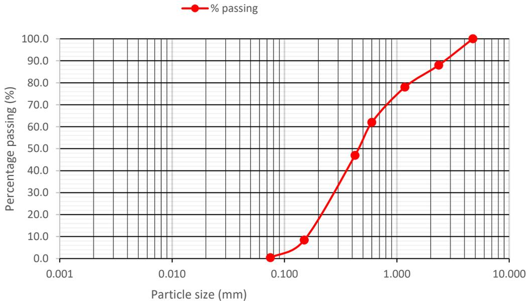
Fig. 1 Particle size distribution of Umuagu studied eroded soil
