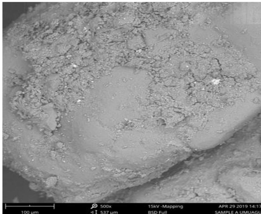
Fig. 5 Scanning Electron Microscopy (SEM) morphology of Umuagu eroded Soil 100μm and 500x exposure
