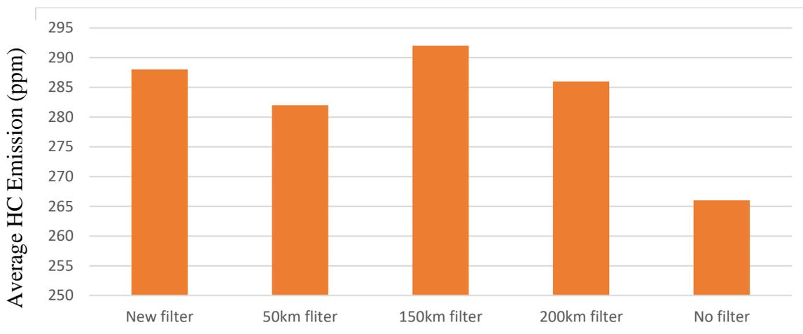
Figure 4: Average HC Emissions (ppm) from New, Used and No Filter Test at High Speed
