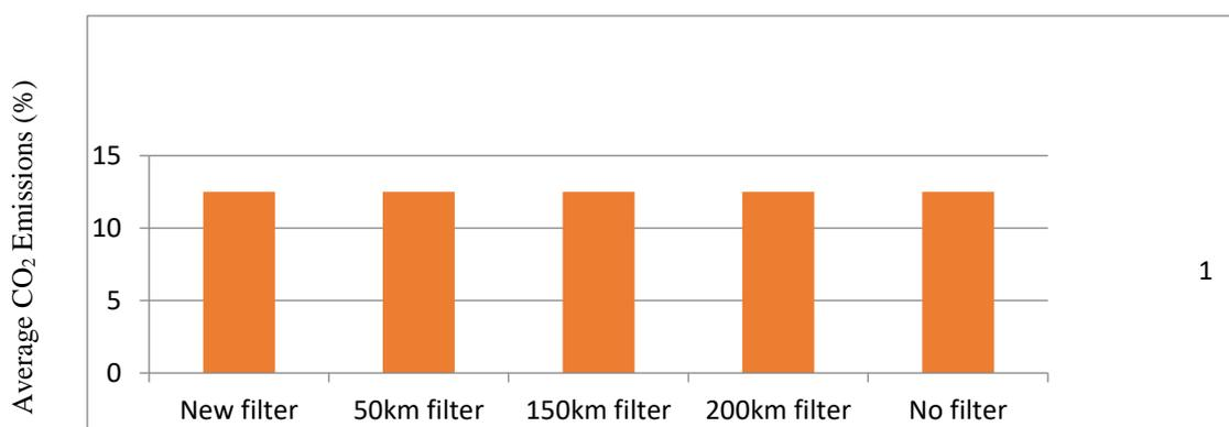
Figure 10: Average CO<sub>2</sub> emissions from new, used and no filter test at high speed
