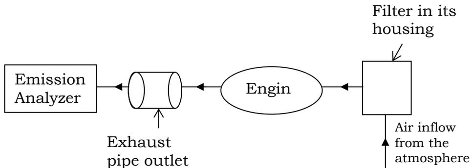
Figure 2: Schematic Diagram of Emission Test
