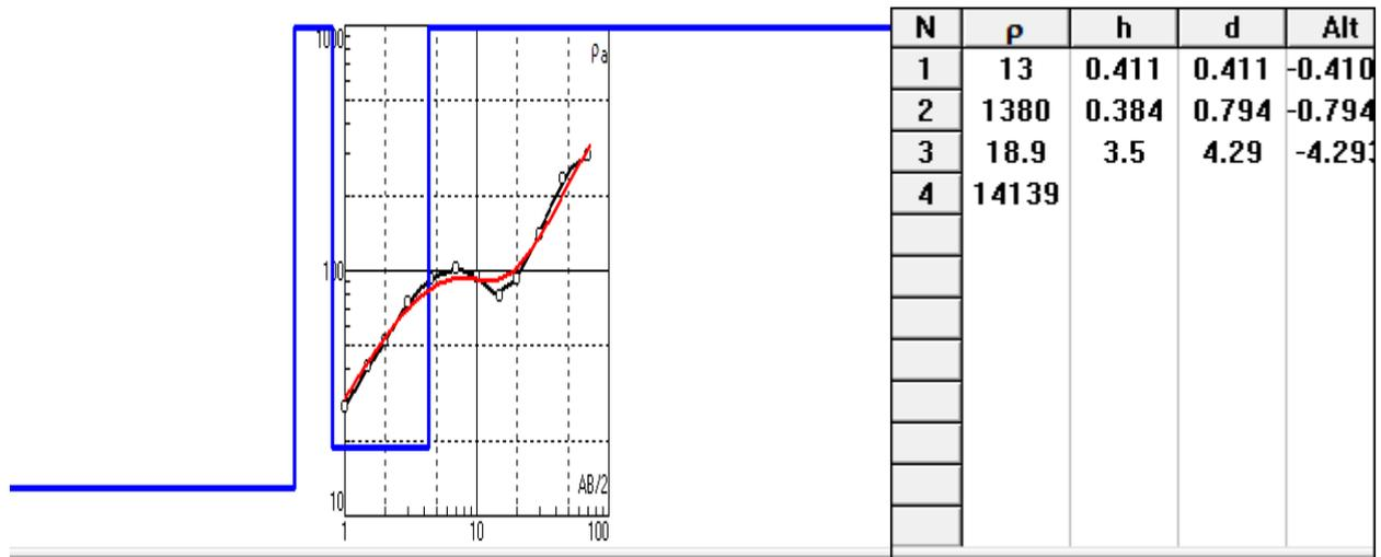
Figure 14. The Sounding curve and interpretation model for VES03 along Profile 3
