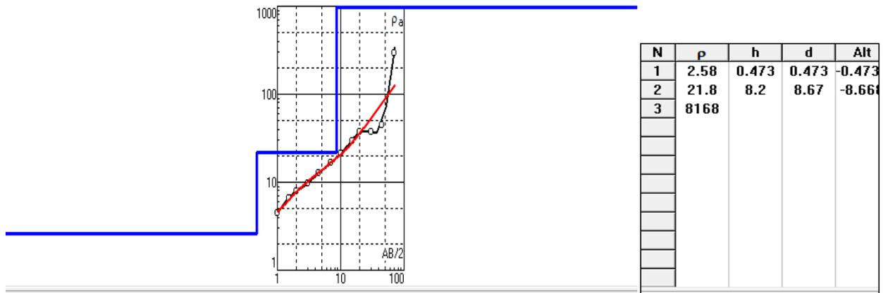
Figure 16. The Sounding curve and interpretation model for VES05 along Profile 3
