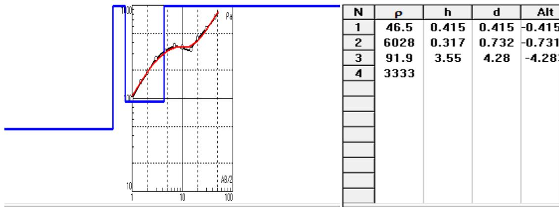
Figure 7. The Sounding curve and interpretation model for VES05 along Profile 1
