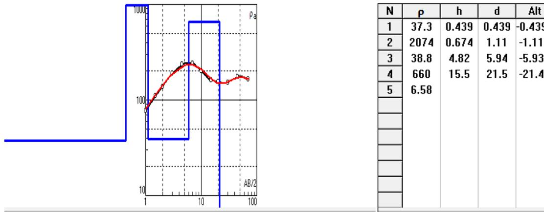
Figure 13. The Sounding curve and interpretation model for VES02 along Profile 3
