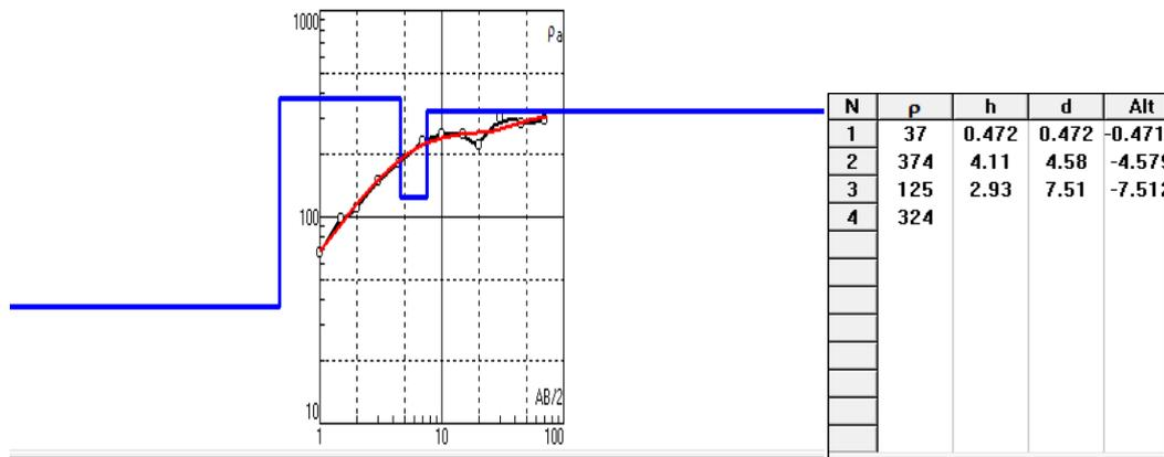
Figure 15. The Sounding curve and interpretation model for VES04 along Profile 3
