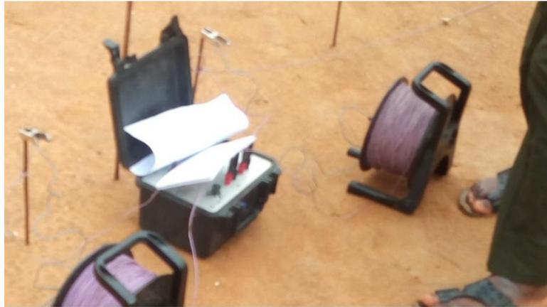
*Plate 1 Terrameter, wire cables and reel*
