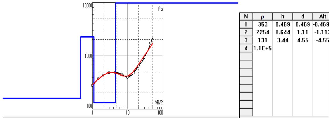
Figure 3. The Sounding curve and interpretation model for VES01 along Profile 1.
