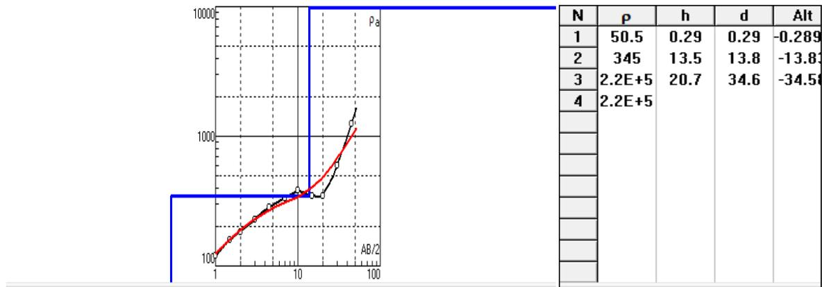
Figure 6. The Sounding curve and interpretation model for VES04 along Profile 1
