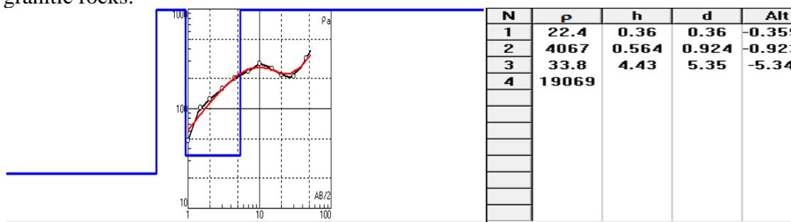
Figure 10. The Sounding curve and interpretation model for VES04 along Profile 2
