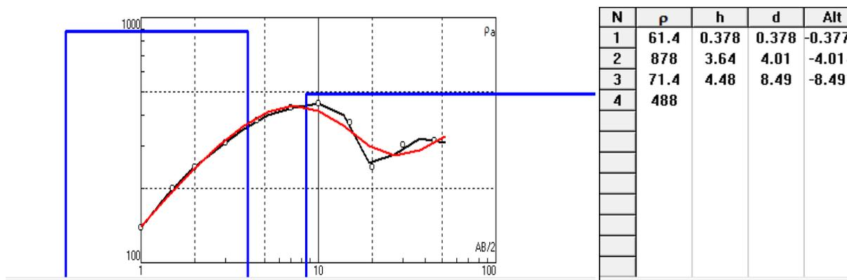
Figure 12. The Sounding curve and interpretation model for VES01 along Profile 3
