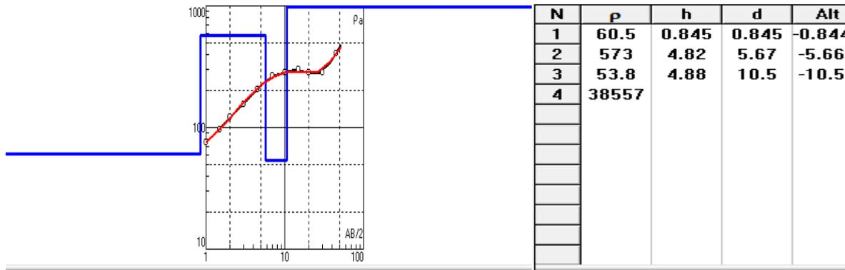
Figure 11. The Sounding curve and interpretation model for VES05 along Profile 2
