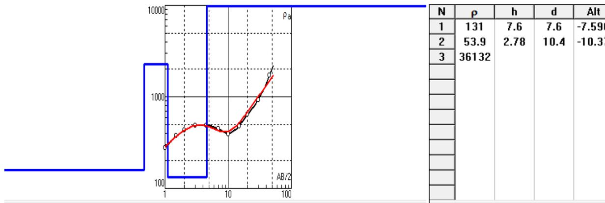
Figure 4. The Sounding curve and interpretation model for VES02 along Profile 1
