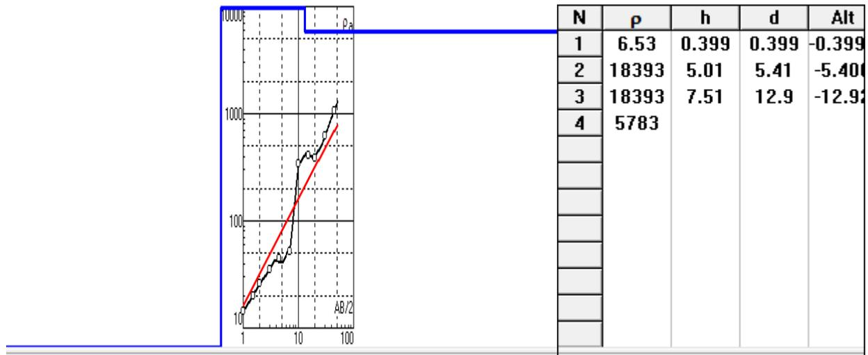
Figure 5. The Sounding curve and interpretation model for VES03 along Profile 1
