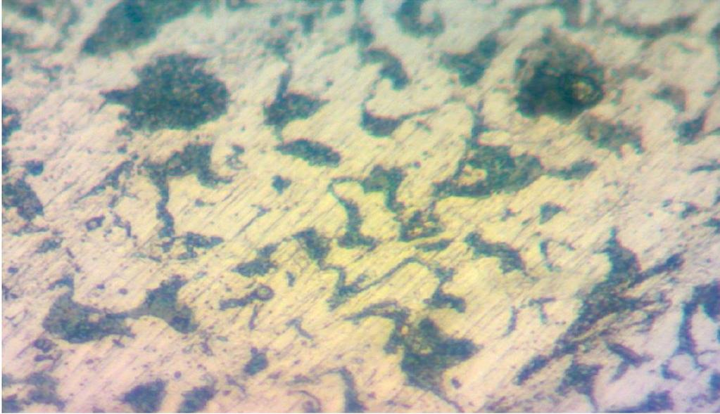
**Plate 1: Micrograph of Low Carbon Steel Specimen (unstrained)**
