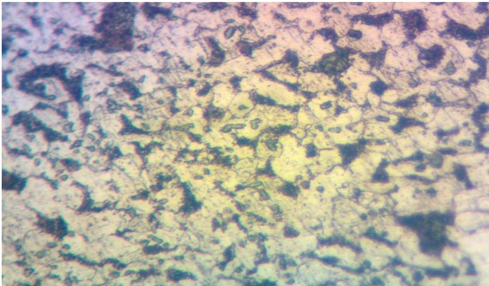
**Plate 4: Micrograph of Low Carbon Steel Specimen (13% Prestrained)**
