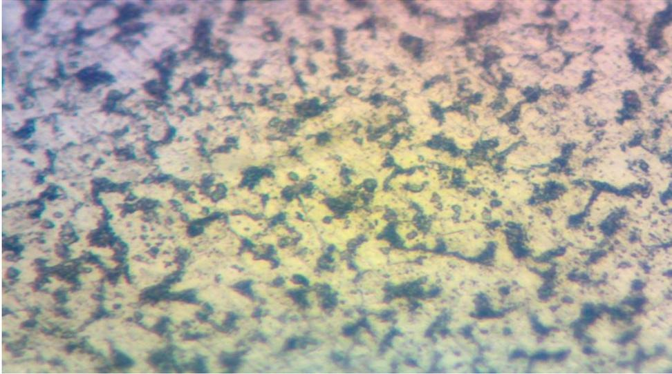
**Plate 5: Micrograph of Low Carbon Steel Specimen (20% Prestraine)**
