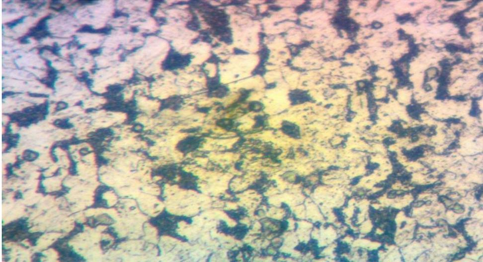
**Plate 3.: Micrograph of Low Carbon Steel Specimen (9% Prestrained)**
