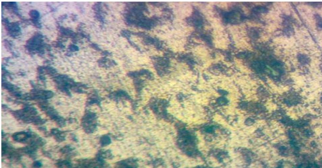
**Plate: 2. Micrograph of Low Carbon Steel Specimen (7% prestrained)**
