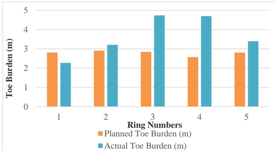
**Figure 5 Planned Toe Burden vs. Actual Toe Burden**
