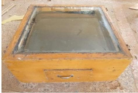
Plate 1. The constructed box-type solar cooker.
