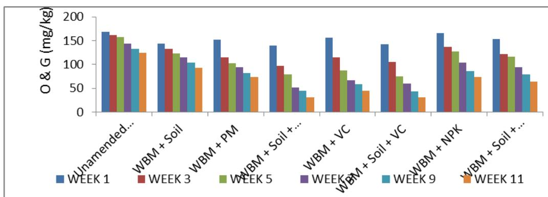
Figure 8: Oil and grease values of compost biotreatment of water based mud
