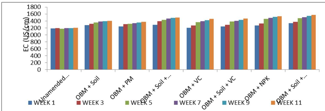
Figure 3: Electrical conductivity values of compost biotreatment of oil based mud
