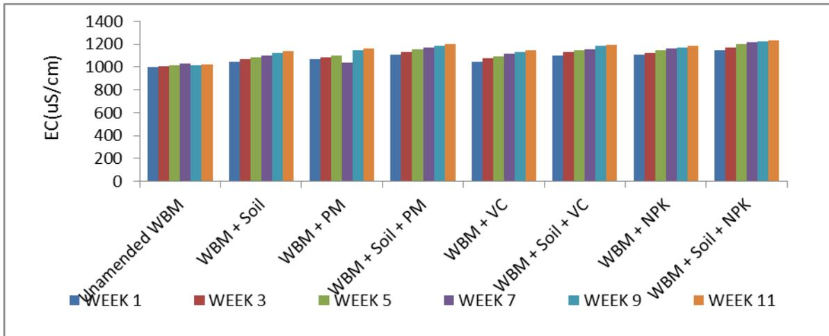
Figure 4: Electrical conductivity values of compost biotreatment of water based mud
