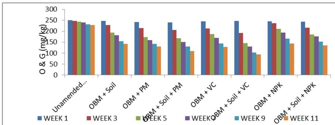
Figure 7: Oil and grease values of compost biotreatment of oil based mud
