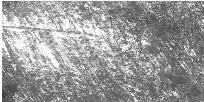
**Plate 4. Micrograph of Test Specimen for High Heat Input (125A) at 200X**
