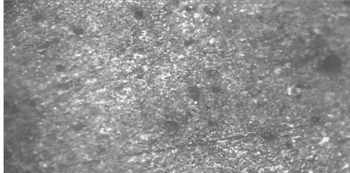
**Plate 3. Micrograph of Test Specimen for Medium Heat Input (112.5A) at 200X**
