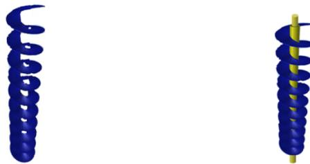
Figure 2: (a) Spiral agitator plate and (b) Assembly of shaft and Spiral agitator plate
