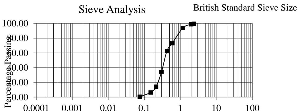
Figure 1: Sieve analysis of fine aggregate
