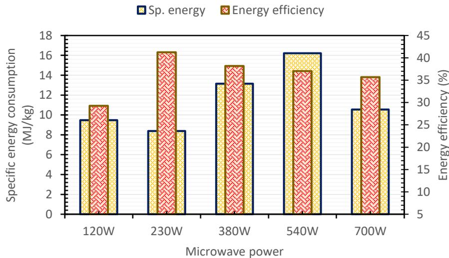
**Figure 12. Mean specific energy consumption and energy efficiency for drying of alligator pepper fruit at varying applied MW-powers**
