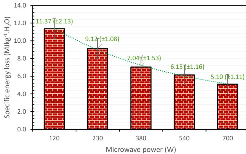
**Figure 11. Variation of specific energy loss with applied MW-power**
