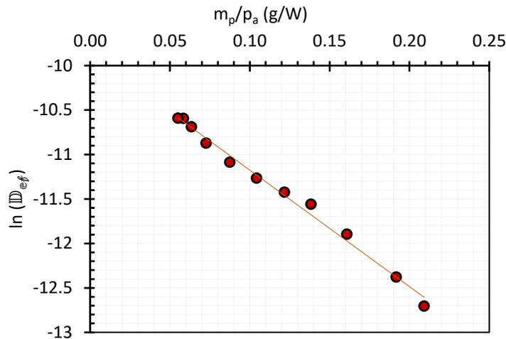
**Figure 8. Correlation between the natural log. of effective moisture diffusion and sample quantity/MW-power for alligator pepper pods**
