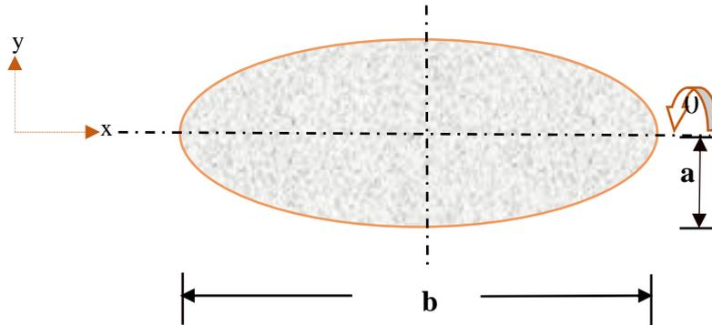
**Figure 2. Schematics of the model geometry for alligator pepper pod rotating about its major axis.**
