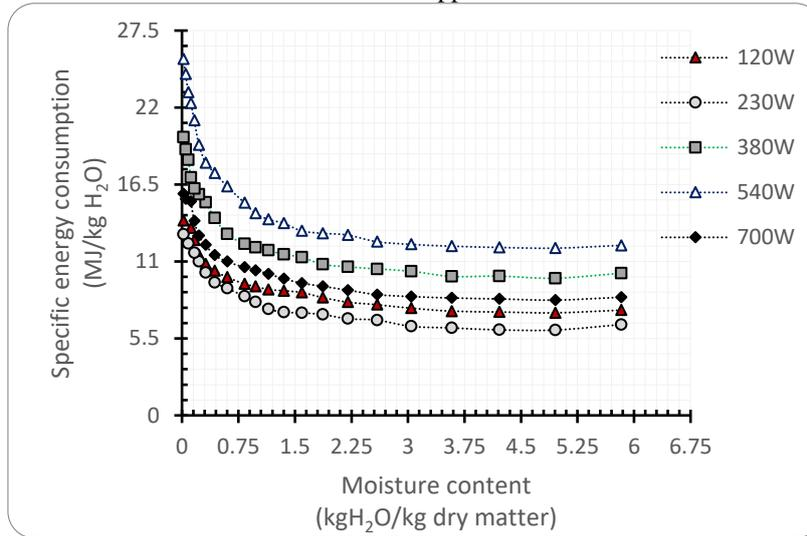
**Figure 9. Effect of moisture content of alligator pepper fruit on the specific energy consumption at varying applied MW-powers**
