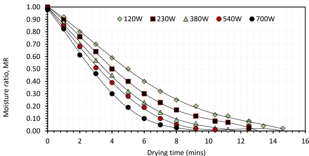
Figure 3. Change in moisture ratio with time of drying at different MW-power levels
