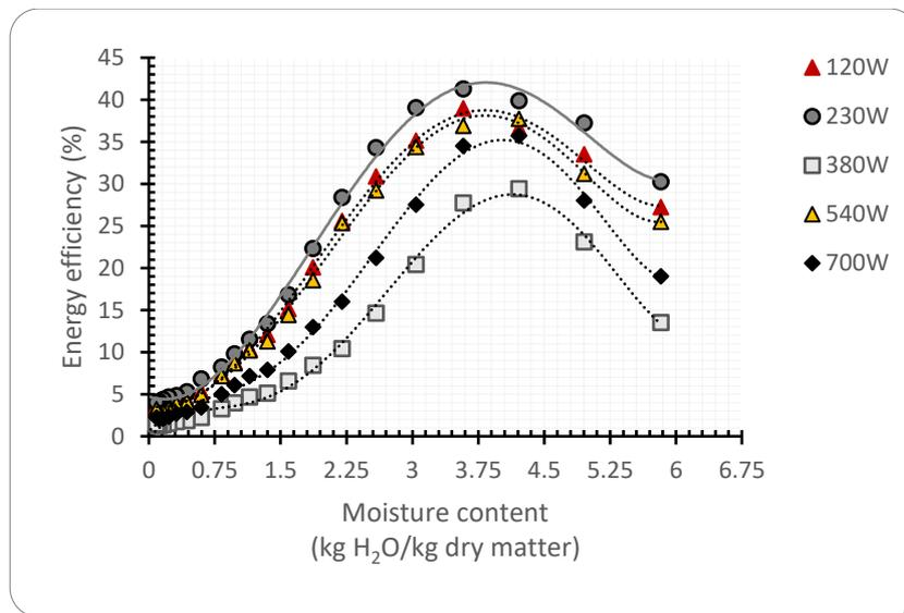
**Figure 10. Change in drying energy efficiency moisture content at different MW-powers**
