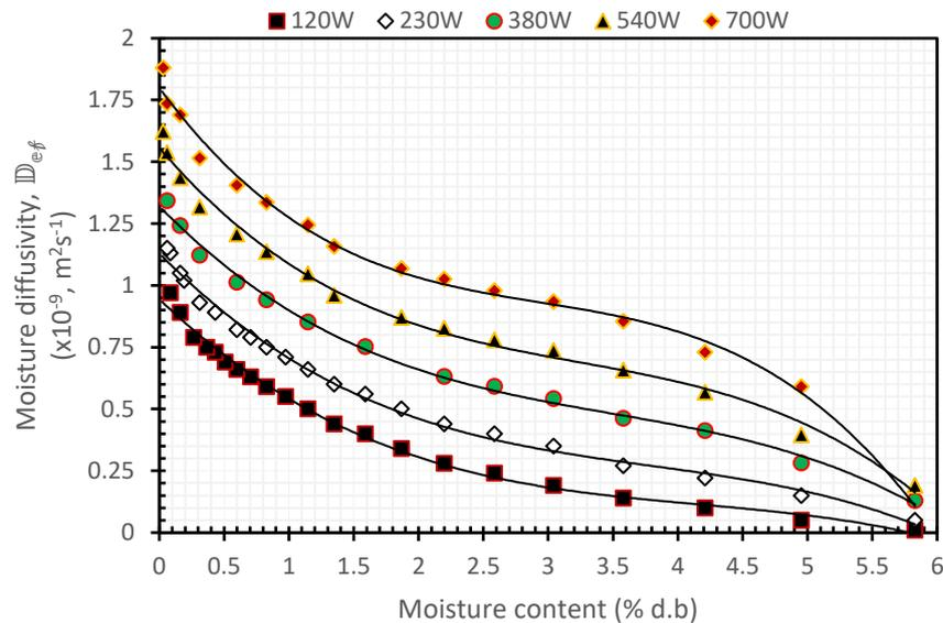
**Figure 7. Effect of sample moisture content on the effective moisture diffusivity at varying MW-power levels.**
