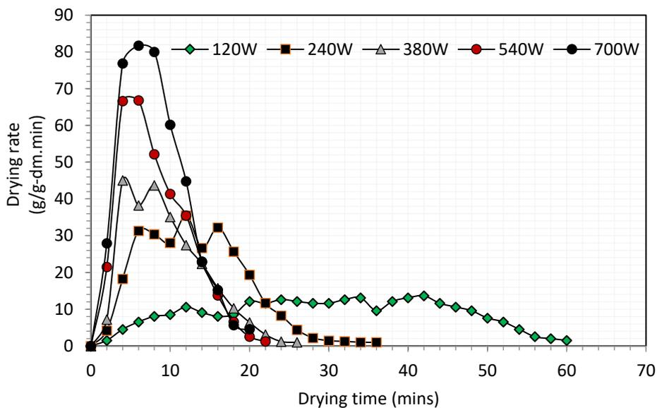
Figure 6. Relationship between drying rate and time at varying applied MW-powers
