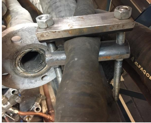
Fig. 2c: Clamp valve and hose
