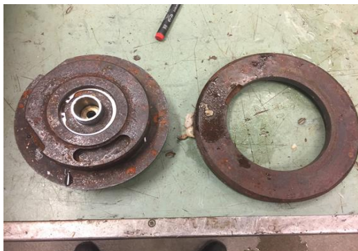
Fig. 4a: Upper shroud of the impeller(L) and insert ring(R) Fig. 4b: Pump housing
