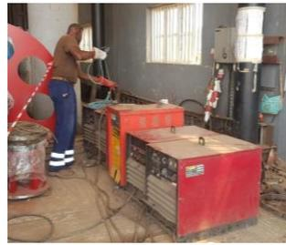
Figure 1:TIG welding equipment
