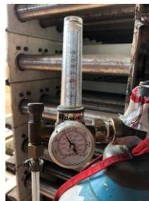
Figure 2:Shielding gas regulator
