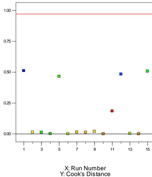
**Figure 8: Plot of Cook's distance versus experimental run order for model representing thickness swelling (continuous bamboo fibre)**
