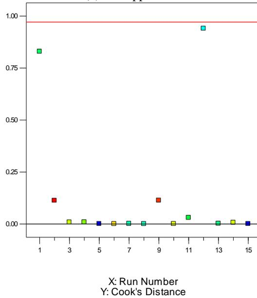
**Figure 7: Plot of Cook's distance versus experimental run order for model representing water absorption (continuous bamboo fibre)**
