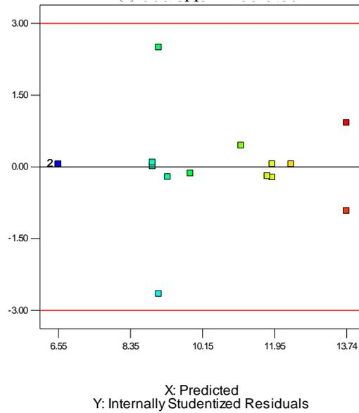
**Figure 3: Plot of residuals versus predicted response for model representing water absorption (continuous bamboo fibre)**
