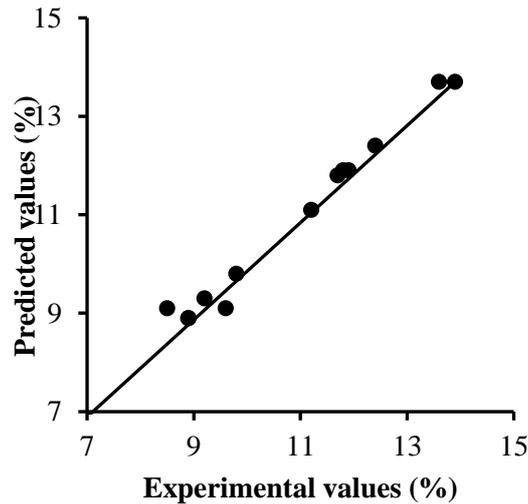
**Figure 9: Parity plot for model representing water absorption (continuous bamboo fibre)**
