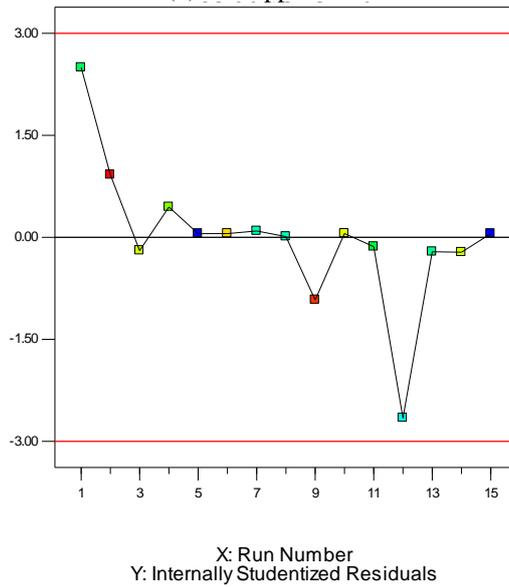
**Figure 5: Plot of residuals versus experimental run order for model representing water absorption (continuous bamboo fibre)**
