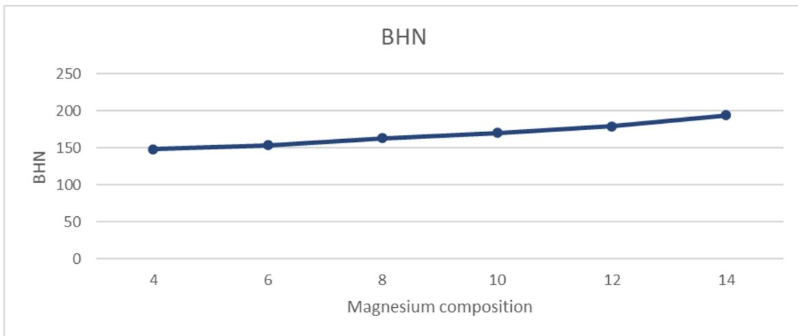
Figure 3. Increasing Hardness with increasing Magnesium Concentration
