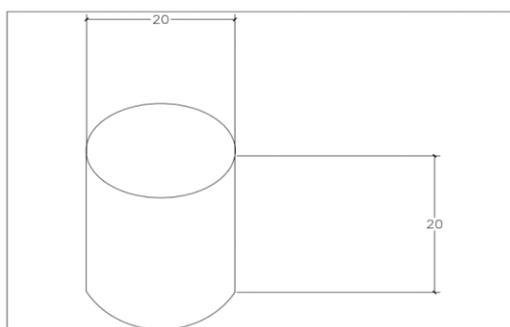
Figure 2: Hardness Test Specimen with diameter in mm
