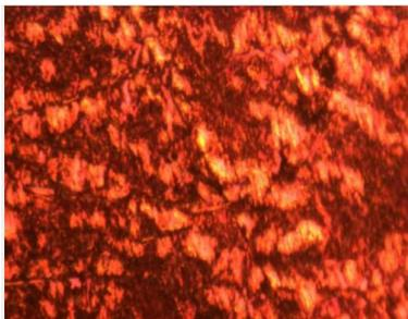
Figure 4. Micrograph of Al-Mg alloy with 14% wt composition of magnesium with 100% magnification
