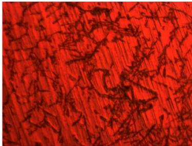
Figure 3. Micrograph of Al-Mg alloy with 8% wt composition of magnesium with 100% magnification
