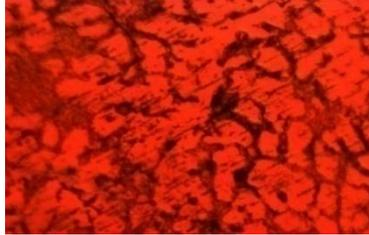
Figure 2. Micrograph of Al-Mg alloy with 4% wt composition of magnesium with 100% magnification
