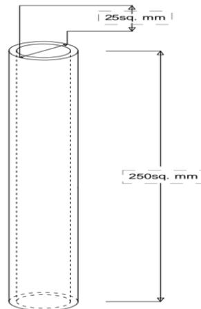
Figure 1. Pattern used for creating the mold
