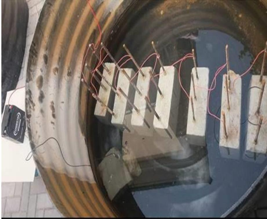
**Figure 2: Picture showing setup for accelerated corrosion experiment**
