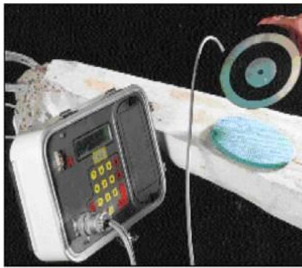
**Figure 3: LPR system for determining corrosion current density**
