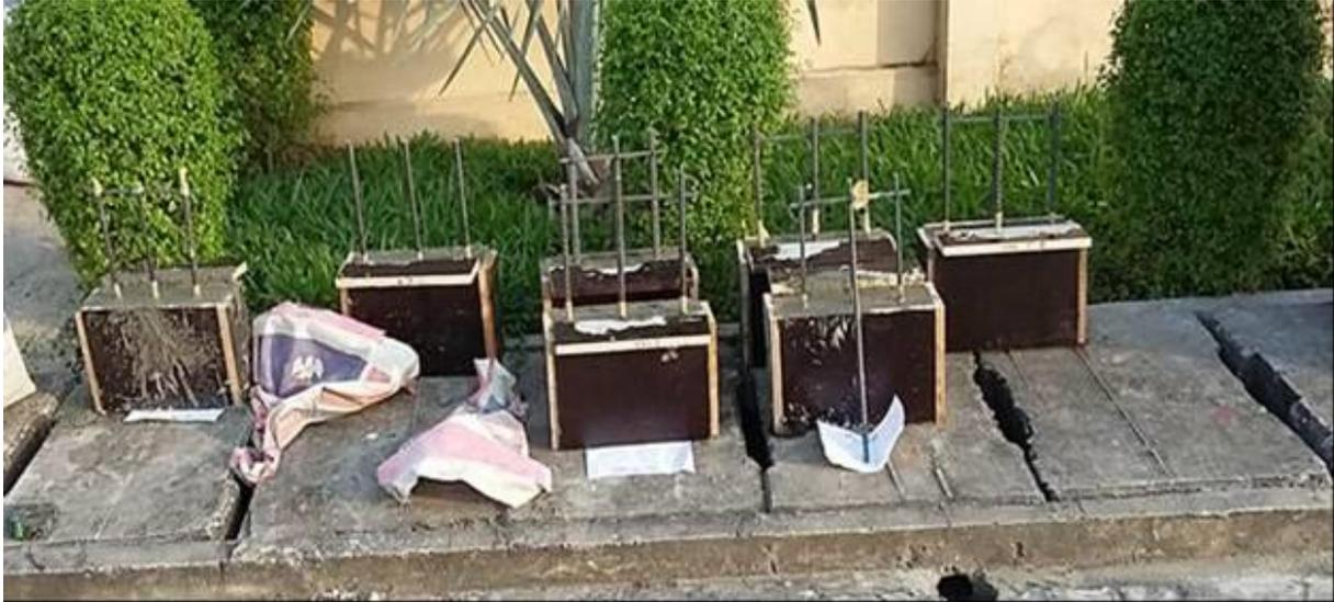
**Figure 1: Cast concrete samples with protruding steel reinforcing bars**
