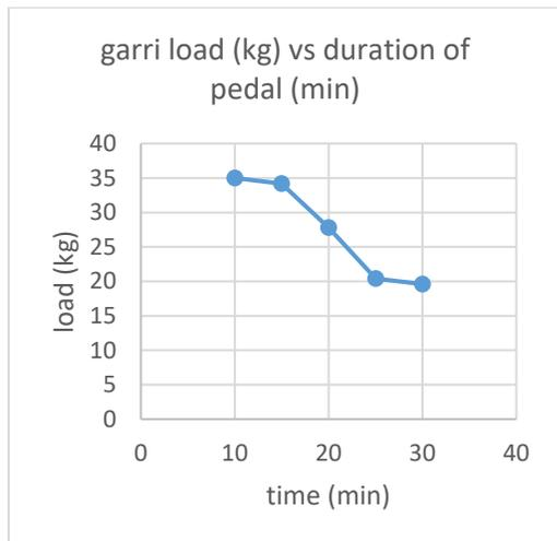
**Figure 6: Graph of Garri Load against Time to Pedal by Male Fryer**
