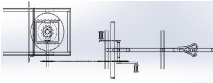
**Figure 2: Plan View of Pedal Operated Garri Frying Mach**
