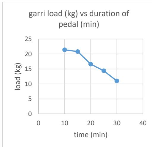
**Figure 7: Graph of Garri Load against Time to Pedal by Female Fryers**
