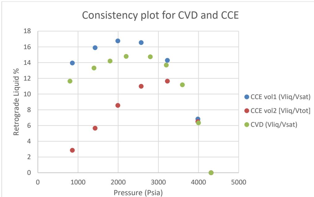
**Figure 4: Liquid dropout from CCE and CVD tests**
