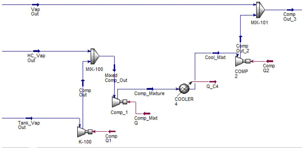
**Figure 7: Process flow diagram for gas compression**
