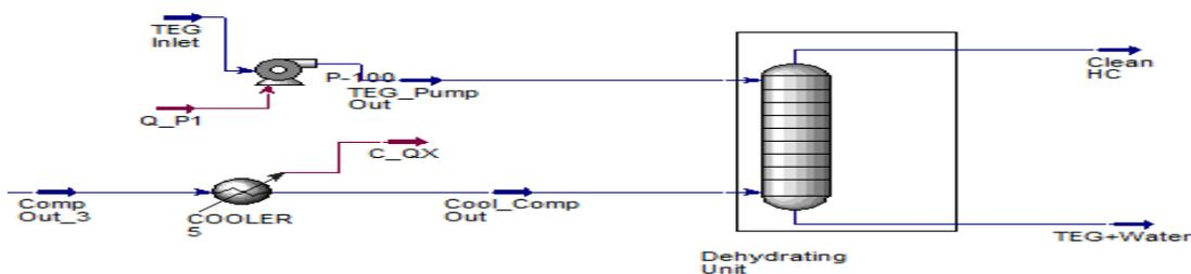
**Figure 8: Process flow diagram for gas dehydration**
