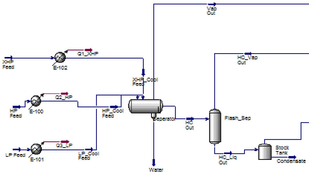
**Figure 6: Process flow diagram showing coolers and separators and condensate tank**
