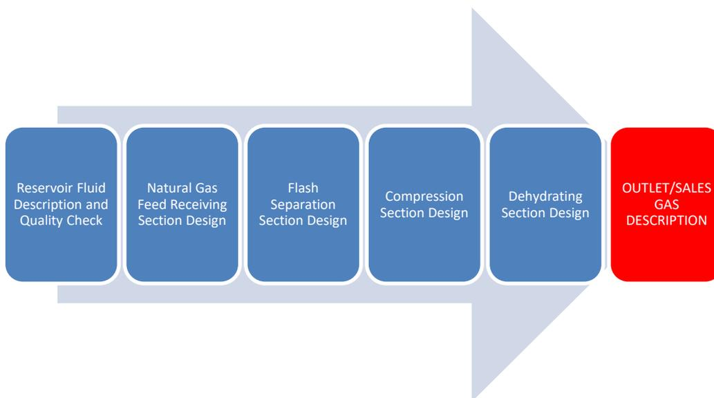
**Figure 1: Various Sections in the Conceptual Design Process**
