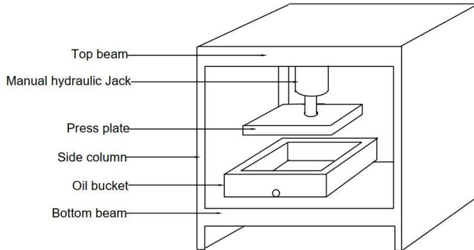
Figure 1. The manual hydraulic oil expeller
