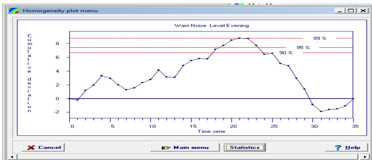
**Figure 2b: Homogeneity test of noise level data (Evening)**
