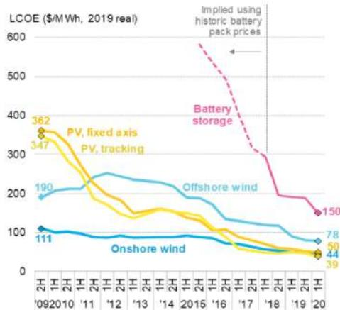
Fig. 5. Global LCOE, 2020 – PV, wind, and battery storage
