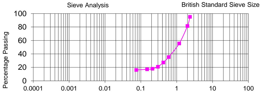
Figure 3: Sieve analysis for the polyethylene (PE) sample
