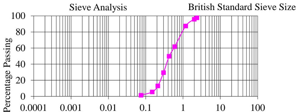
Figure 2: Sieve analysis for the fine aggregate
