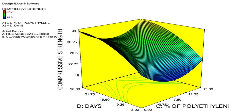
Figure 6: Compressive strength and percentages of PE additive 3D graph
