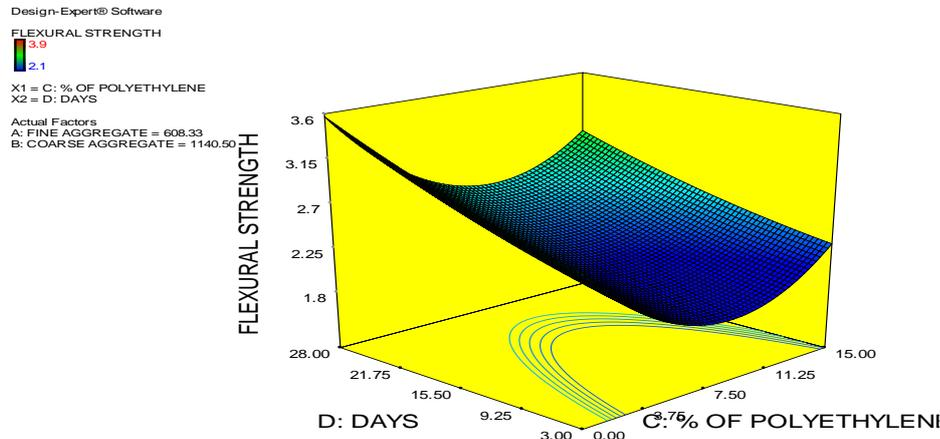
Figure 7: Flexural strength and percentages of PE additive 3D graph
