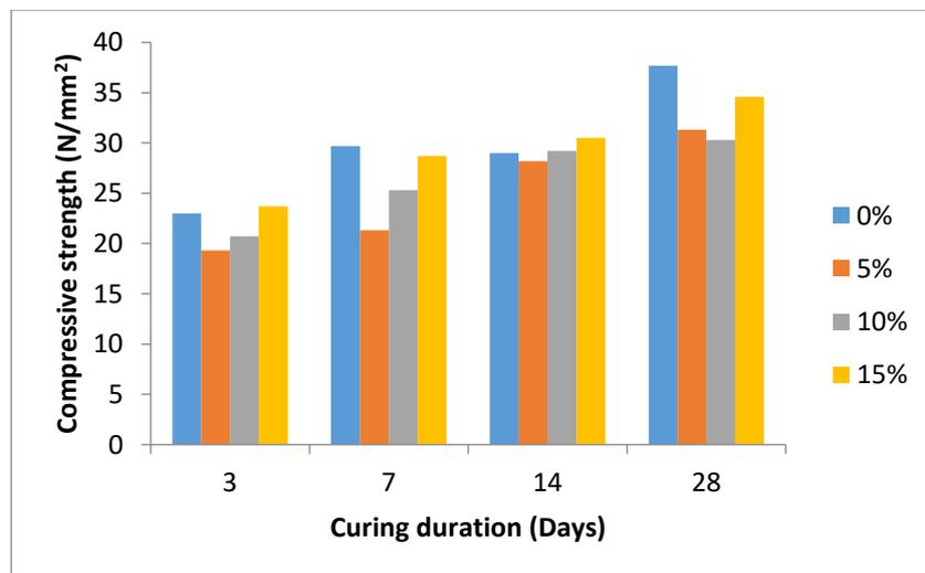
Figure 4: Compressive strength and percentages of PE additive graph
