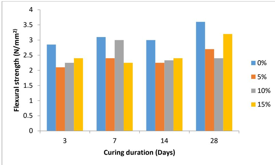
Figure 5: Flexural strength and percentages of PE additive graph
