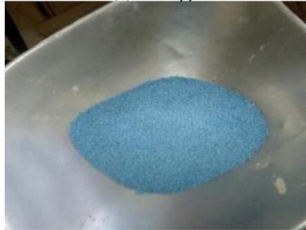
Figure 1: Pulverized polyethylene (PE) sample
