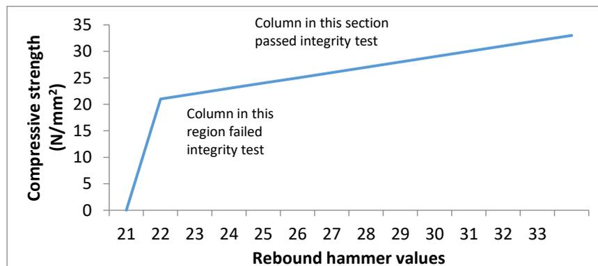
Figure 1: Graph of compressive strength against rebound value for partly failed columns
