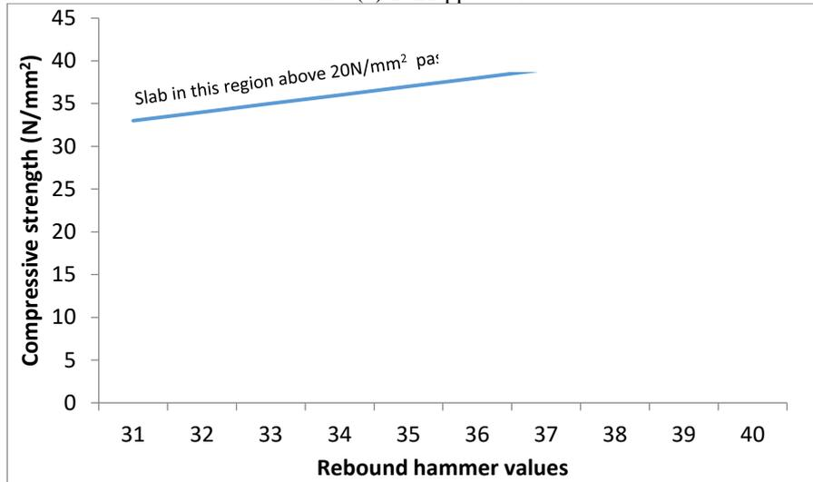
Figure 2: Graph of compressive strength against rebound value for ground floor concrete slab
