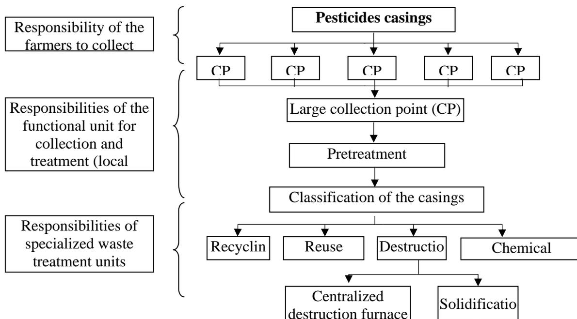
**Figure 9. Schematic diagram of pesticide waste management model**
