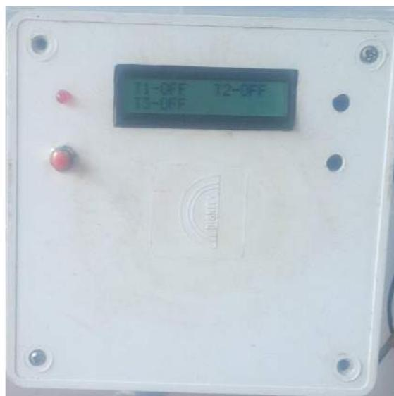
**Figure 5. Central node with state of three valves (T1-T3) displayed on LCD**
