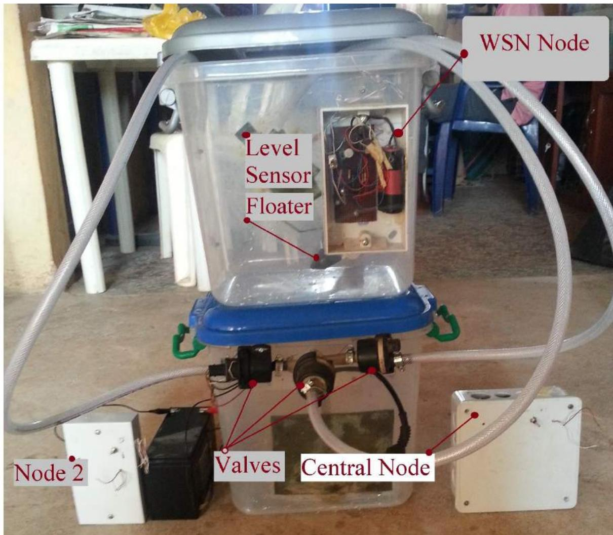
Figure 4. Prototype showing a central node, 2 remote nodes and 3 valves
