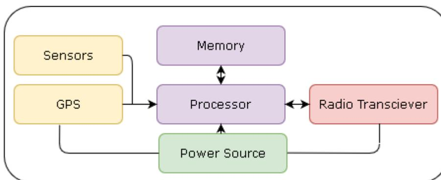
**Figure 1: Components of Wireless Sensor Network Node**
