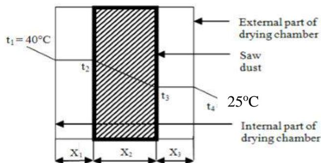
Figure 3. Insulation of drying chamber using saw dust
