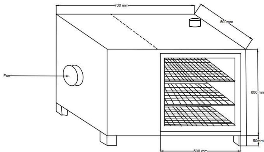
Figure 2. Diagram showing the grain dryer.
