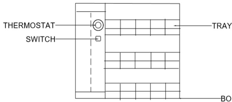
Figure 1. Diagram showing the arrangement of the trays in the drying chamber
