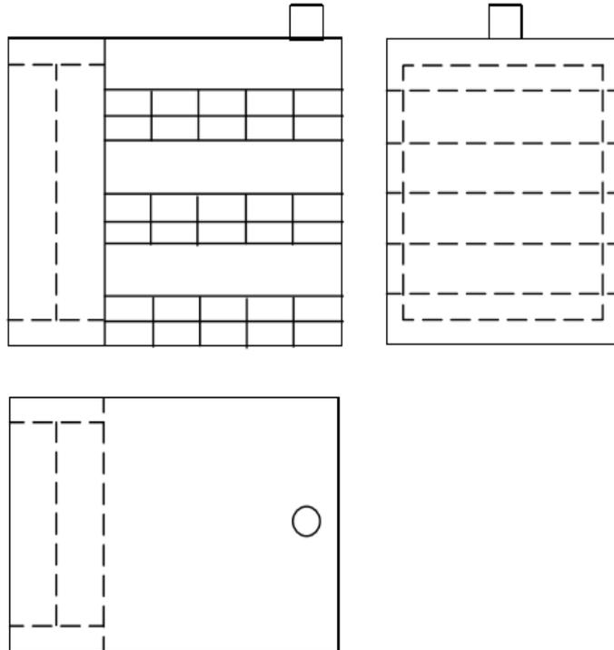
First angle orthographic projection of the portable grain dryer
