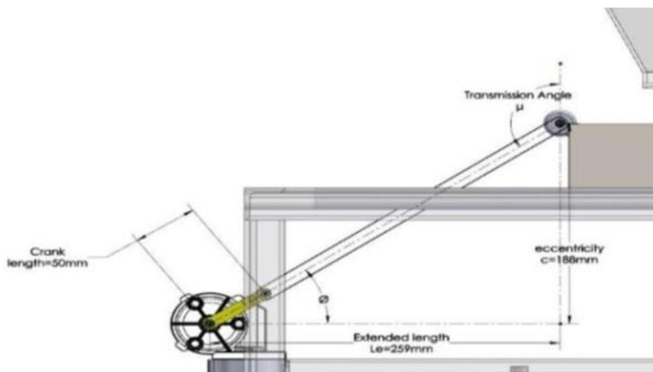
Figure 2a: An extended dead center position of the connecting rod
