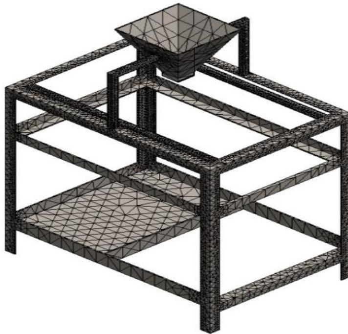
Figure 3: Mesh model of the frame structure of the sand sieving and heating machine
