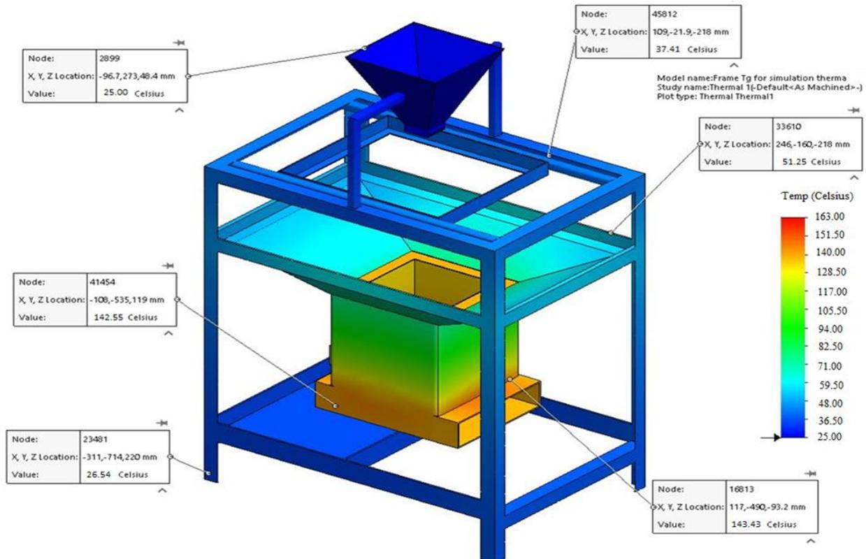
Figure 11: Simulation result for steady state heat transfer analysis of the sand sieving and heating machine
