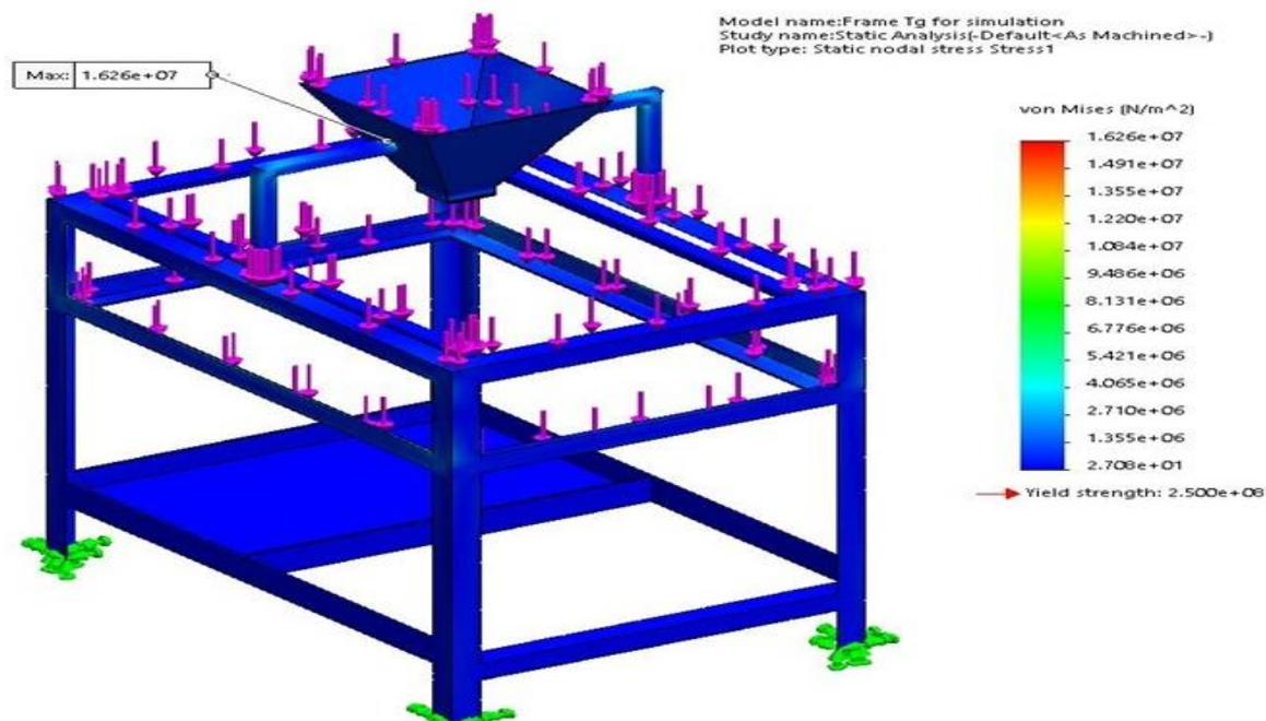
Figure 9: Simulation for static modal stress distribution
