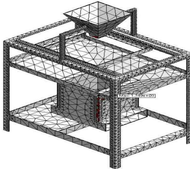
Figure 4: Mesh model for thermal analysis of the sand sieving and drying machine
