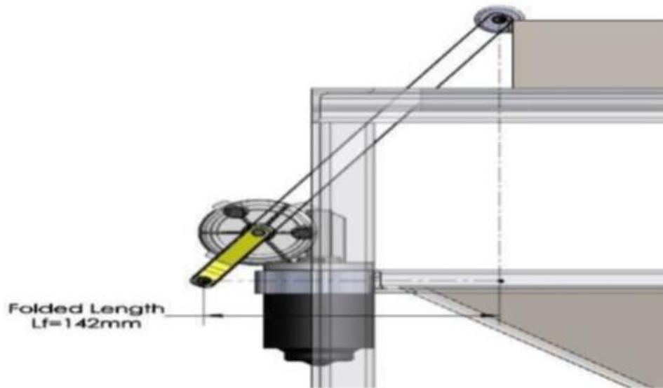
Figure 2b: The folded Dead center position with the connecting rod
