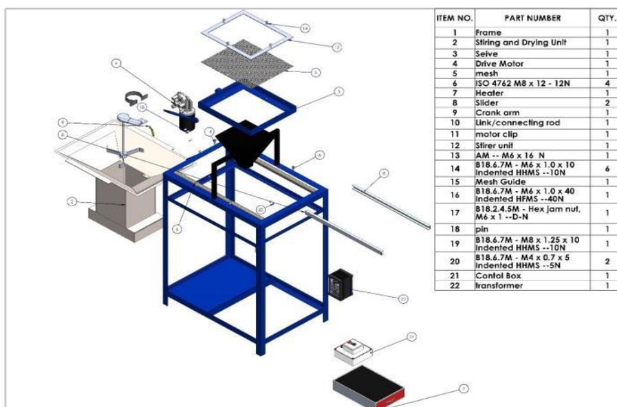
Figure 5: An exploded view of the sand sieving and drying machine
