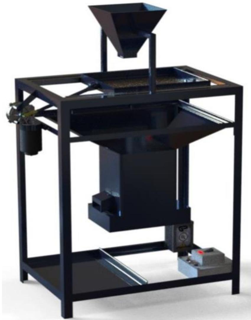
Figure 6: An isometric view of the sand sieving and drying machine
