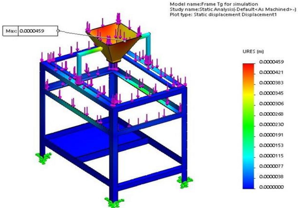
Figure 10: Simulation for static displacement
