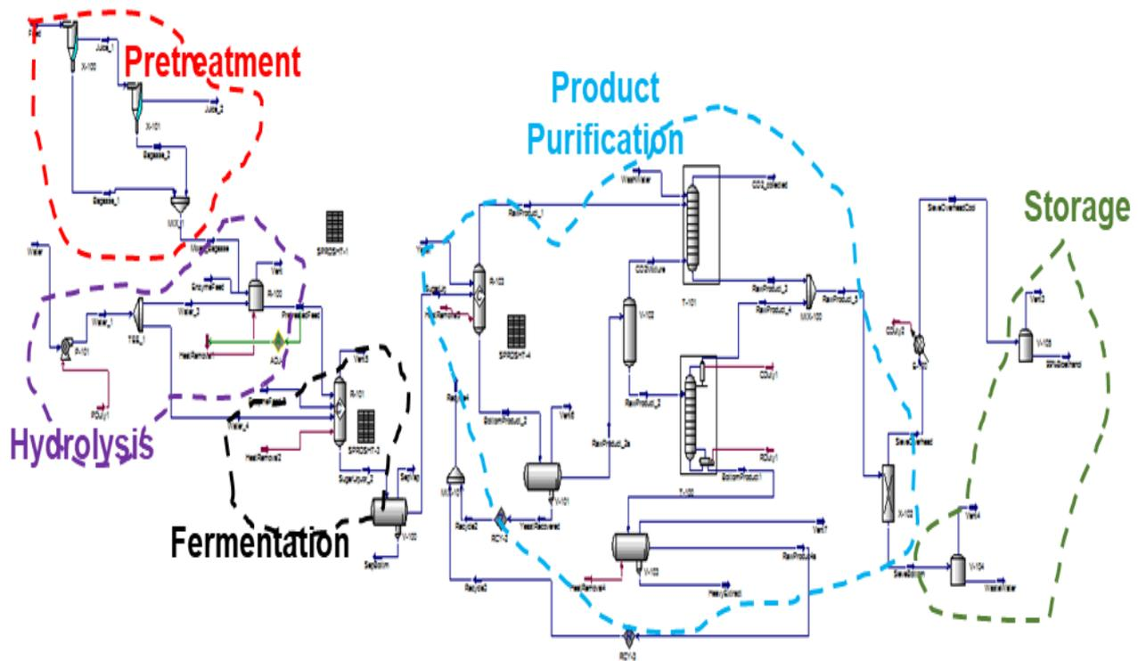
**Figure 2:** PFD for Bioethanol Production from Sorghum Bagasse
