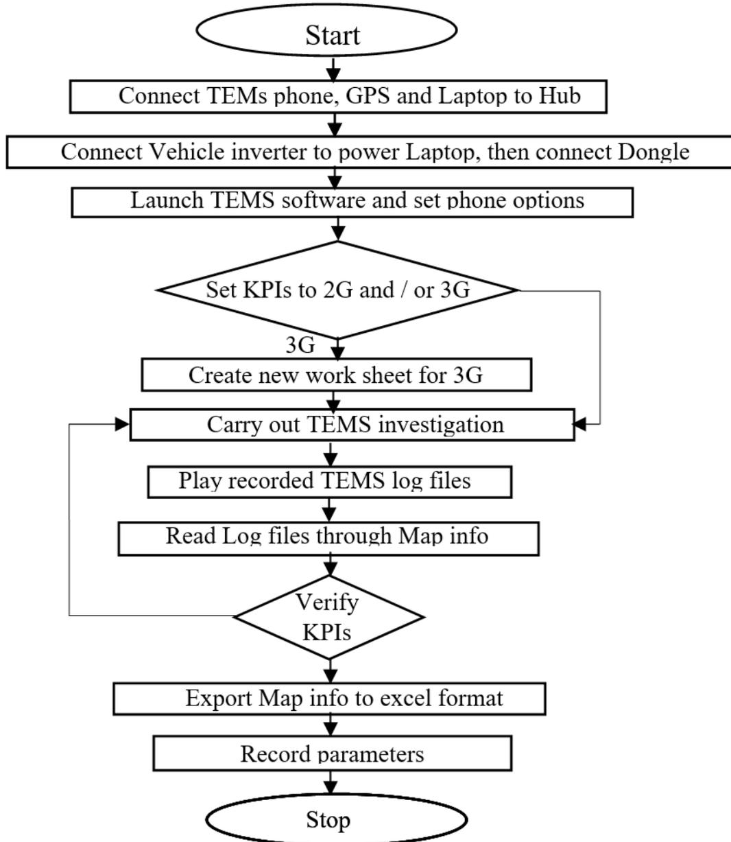
Figure 1: Flow chart for the Drive Test
