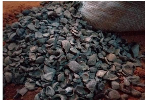
**Figure 3.0:** Crushed Palm Kernel Shell Sample
