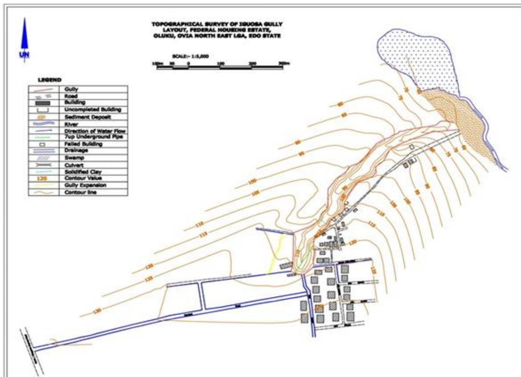
Figure 2: Topographical survey of Iguosa Gully, Benin City
