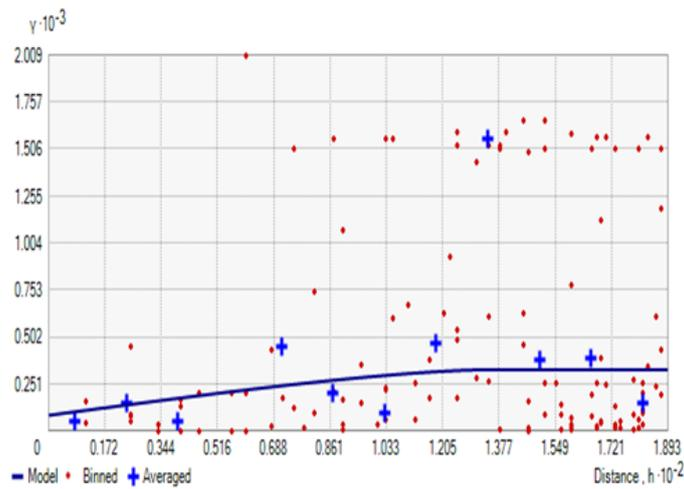
Figure 8: Cohesion semi-variogram
