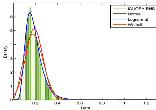
Figure 11: Probability Density Frequency of FOS of Iguosa Gully (RHS)
