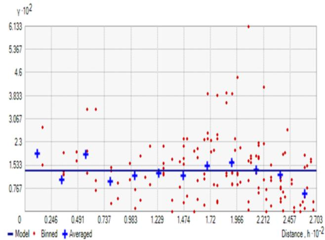
Figure 7: Specific gravity semi-variogram
