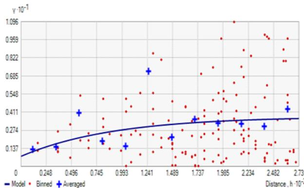
Figure 6: Optimum moisture content semi-variogram
