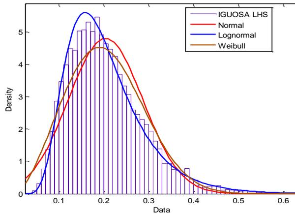
Figure 10: Probability Density Frequency of FOS of Iguosa Gully (LHS)
