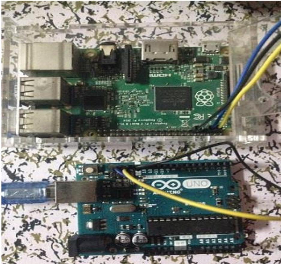
Figure 10: I<sup>2</sup>C communication between Raspberry Pi and Arduino
