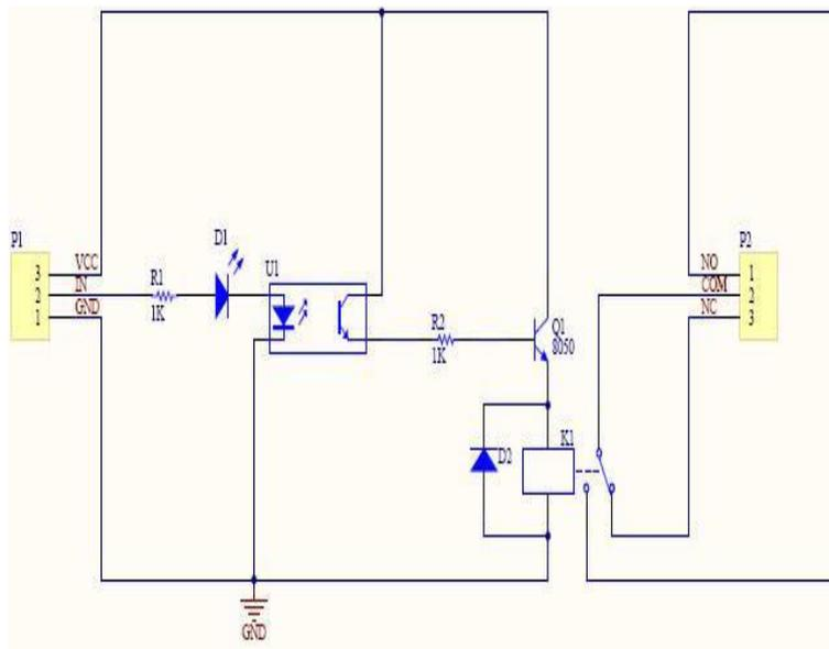
Figure 4: Relay Module
