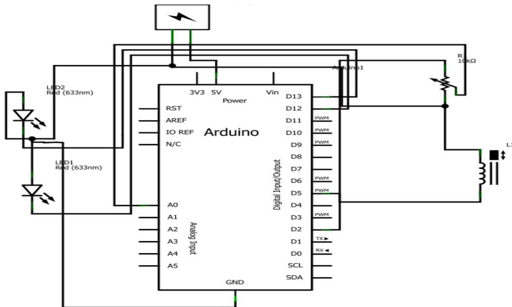
Figure 8: Arduino UNO R3 Pinout Allocation
