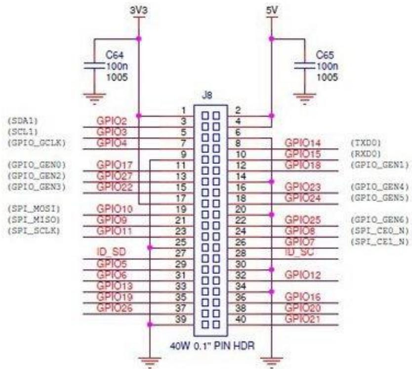
Figure 7: Raspberry Pi 2 Model B Pinout Allocation
