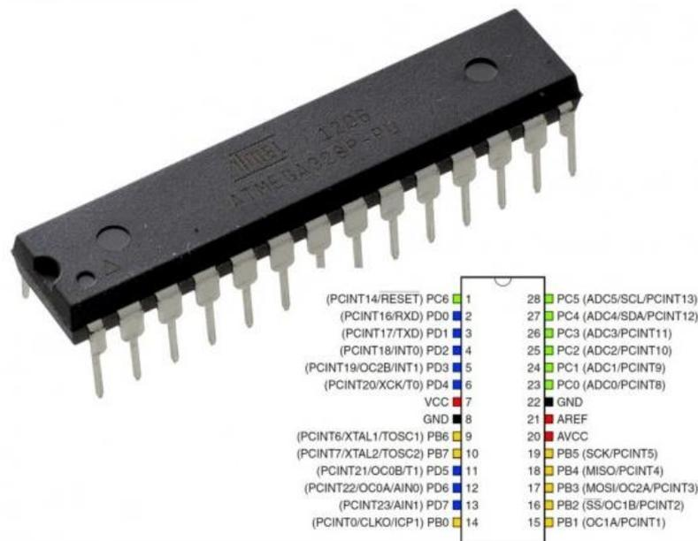
Figure 3: ATmega328 Microcontroller
