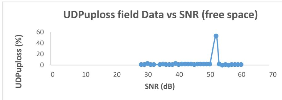
Figure 3: Average UDPuploss field Data vs SNR (free space)
