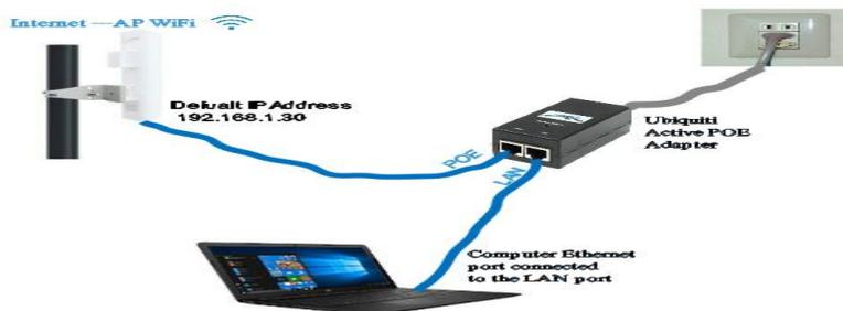
Figure 2: Experimental setup with a connected ethernet user
