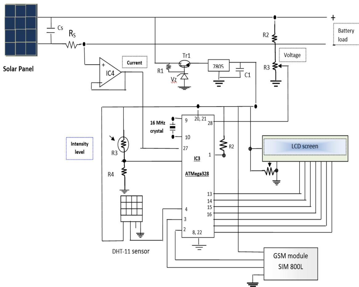
Figure 5: Complete circuit diagram of the IOT based Datalogger.
