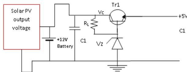
Figure 3: Power supply circuit
