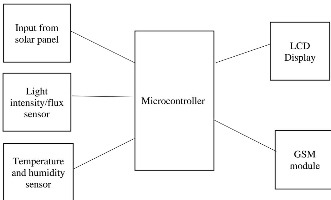
Figure 2: Block diagram of an IoT-based datalogger.
