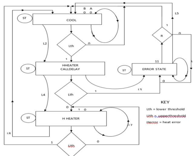
**Figure 3:** ASM Chart for Temperature Control System
