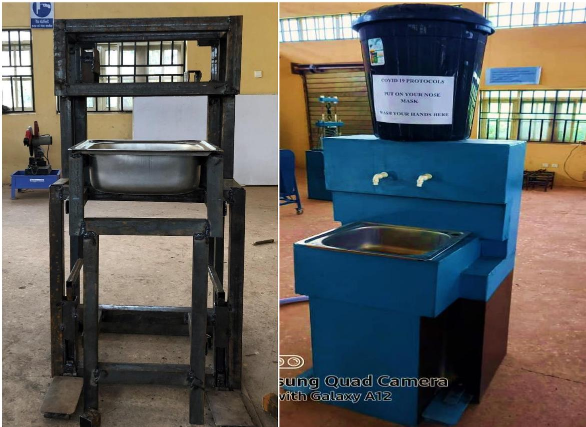
**Fig 4:** The skeletal frame and fully installed views of the Dispenser during Fabrication
