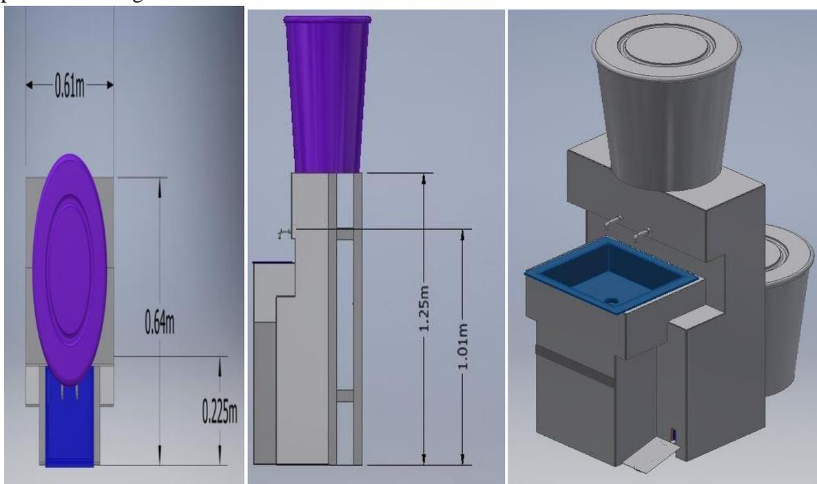
**Fig. 1:** Top, Side, and Isometric Views of the Dispenser
