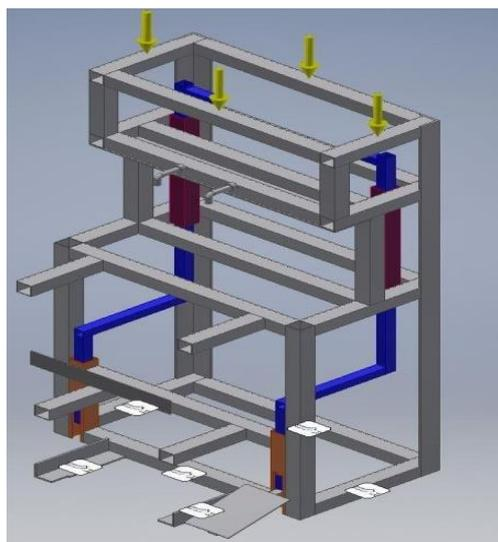
**Fig.3:** Direction of Applied Force (Load) on Machine
