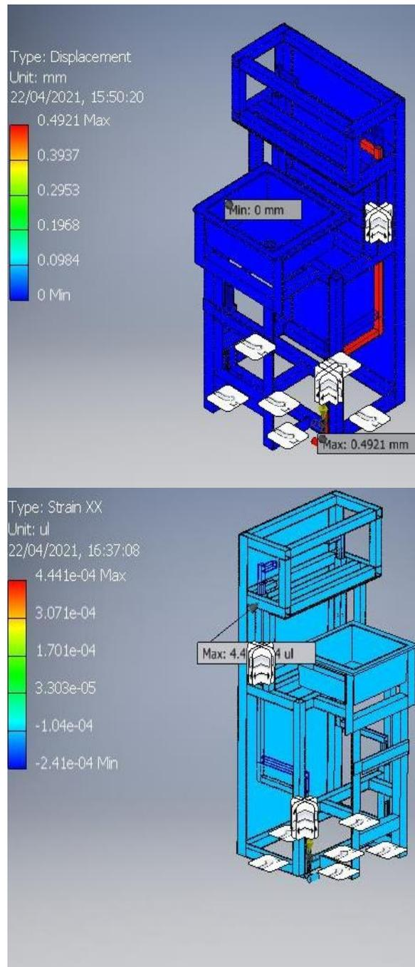
(a) Maximum displacement      (b) Maximum strain
