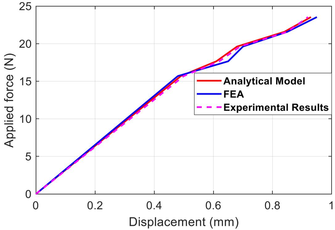
Fig. 6. Force-Displacement relationship for water dispenser
