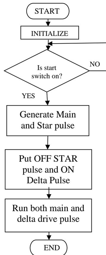
Figure 1. Flowchart for ATMEGA328P control sequencer codes
