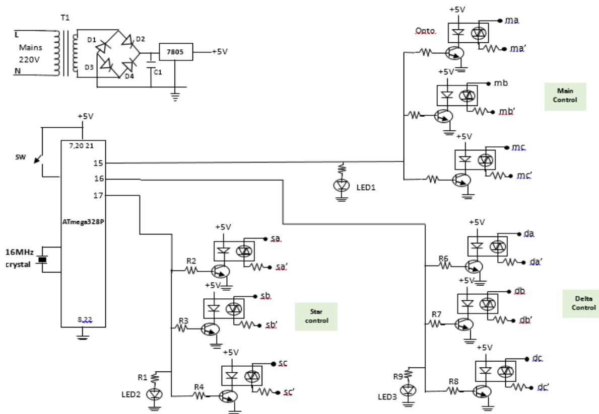
Figure 5: Star-Delta starter Control Circuitry
