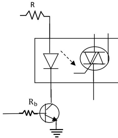
Figure 3. Optocoupler/Transistor circuit
