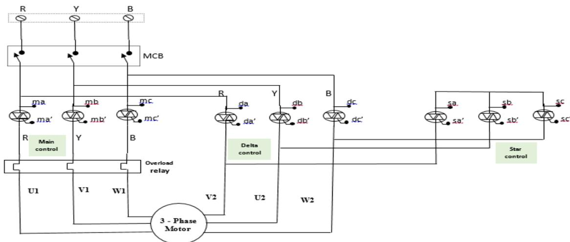
Figure 6: power TRIAC Star – Delta Starter Circuit
