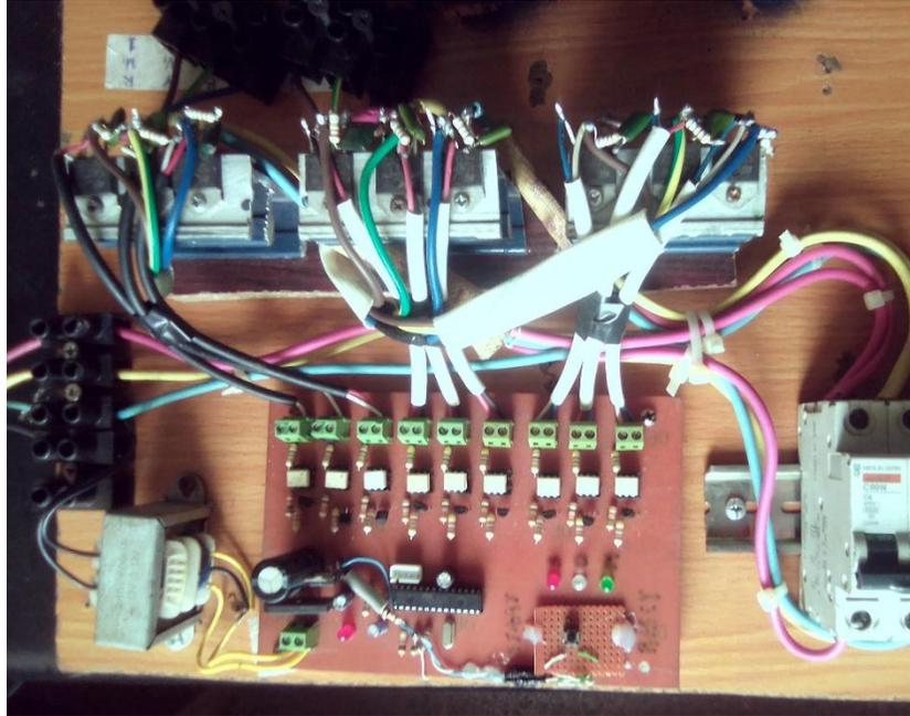
Figure7: Pictorial view of the implemented Solid state star – delta starter
