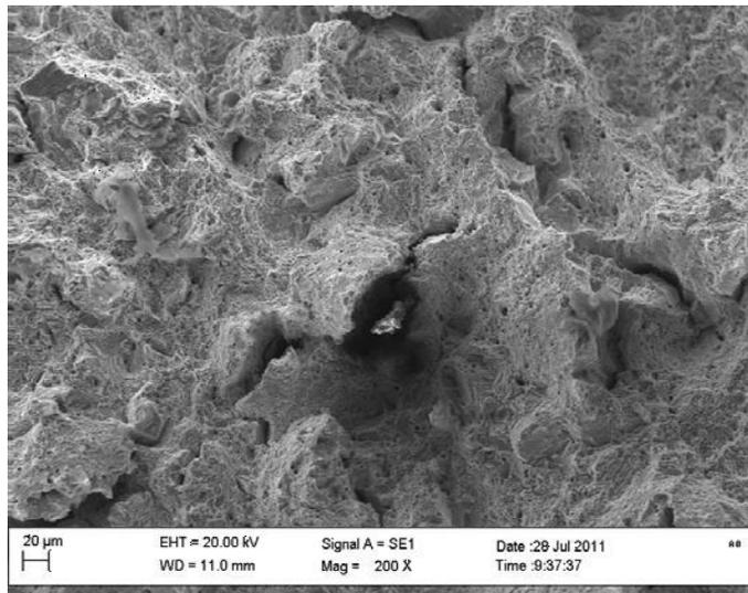
**Figure 7:** Fracture surface of AISI 1040 steel austenised at 1030<sup>0</sup> C
