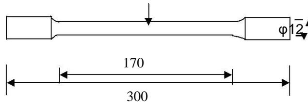
Figure 1. Tensile test sample
