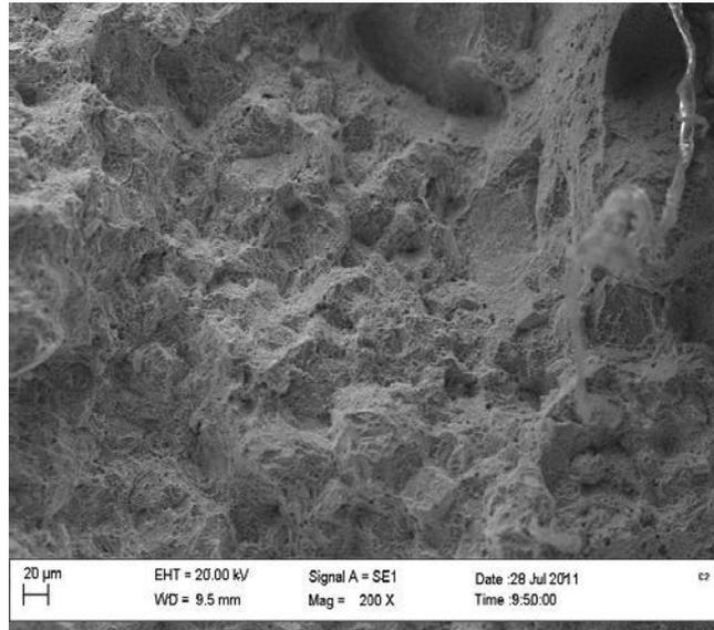
**Figure 6:** Fracture surface of AISI 1040 steel austenised at 830<sup>0</sup> C
