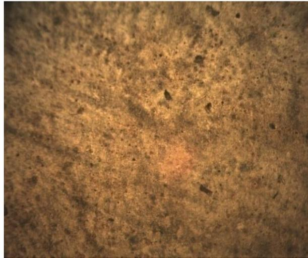
**Figure 4:** Microstructure of AISI 1040 steel austenised at 1030<sup>0</sup>C
