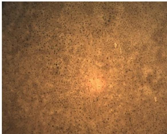
**Figure 3:** Microstructure of AISI 1040 steel austenised at 830<sup>0</sup>C
