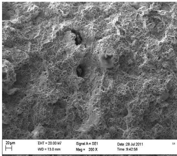
**Figure 5:** Fracture surface of AISI Steel that was not austenised
