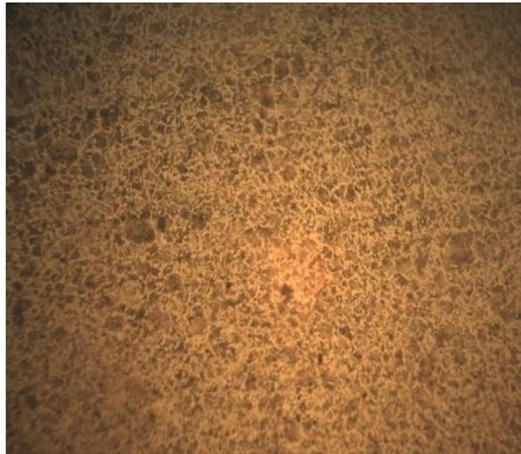
**Figure.2:** Microstructure of AISI 1040 steel that was not austenised
