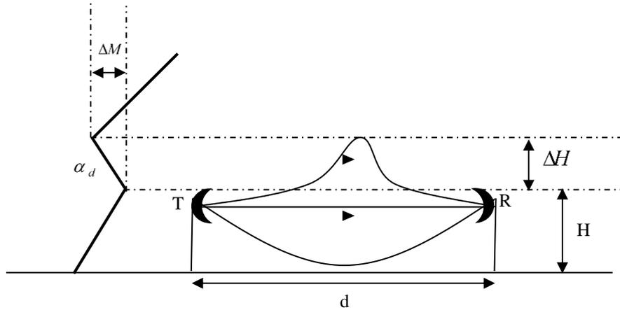
Figure 1: Schematic Description of Ducting phenomenon with Transmitter (T), Distance (d), Receiver (R)
