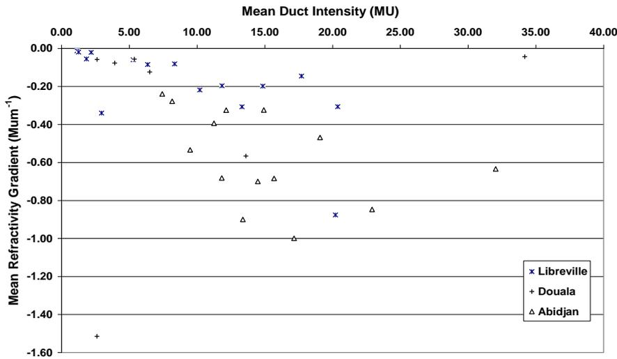
Figure 2: Mean Refractive Gradient and Mean Duct Intensity
