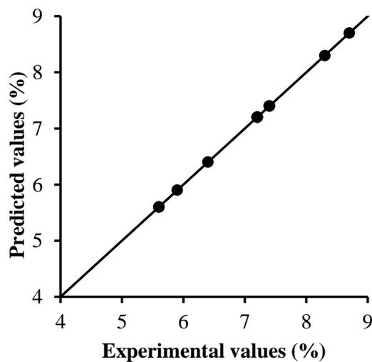
Figure 4: Parity plot for model representing water absorption.
