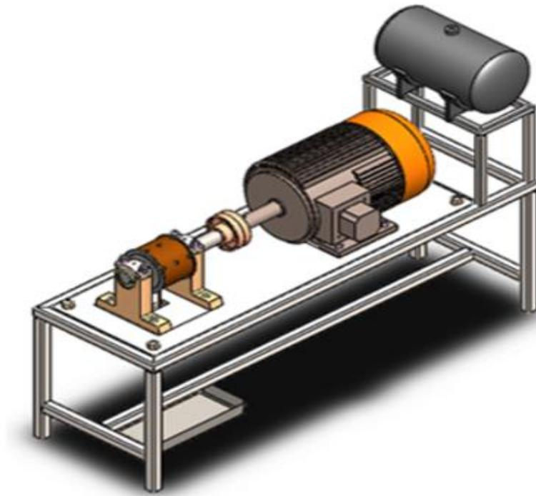
Figure 3. Isometric view of the journal bearing test rig
