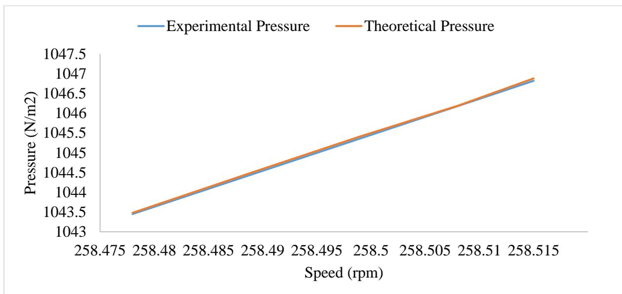
Figure 6. Graph of journal bearing speed against pressure generated
