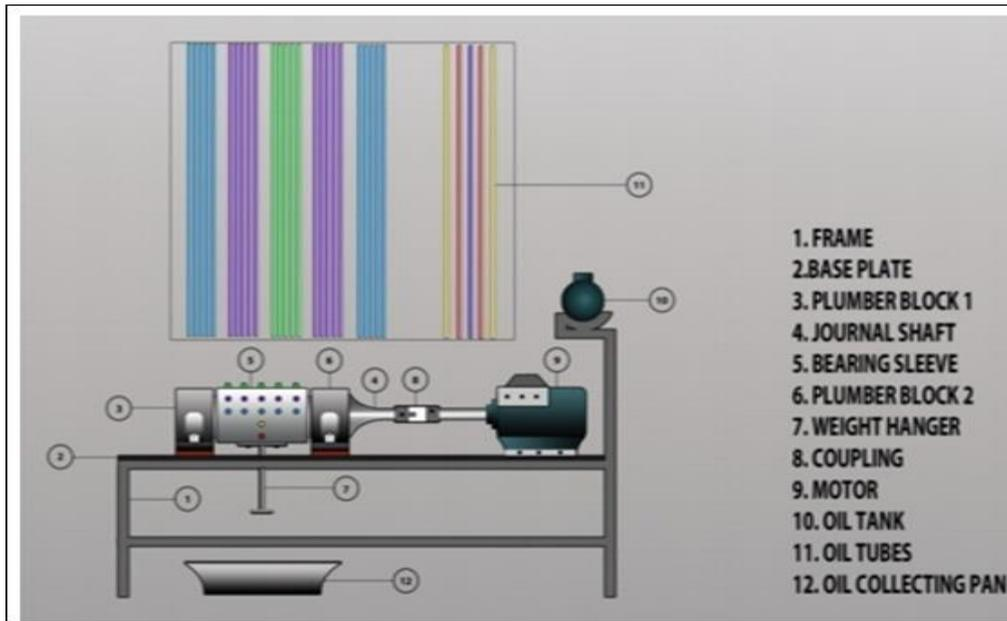
Figure 1. Isometric view of first design concept
