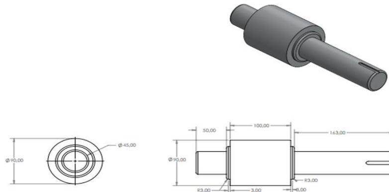
Figure 4. Dimensioned view of the bearing test rig shaft
