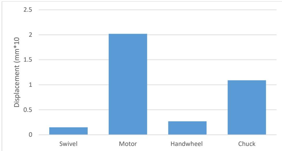
Figure 1: Measured values of amplitudes at different points in the drilling machine at no-load condition
