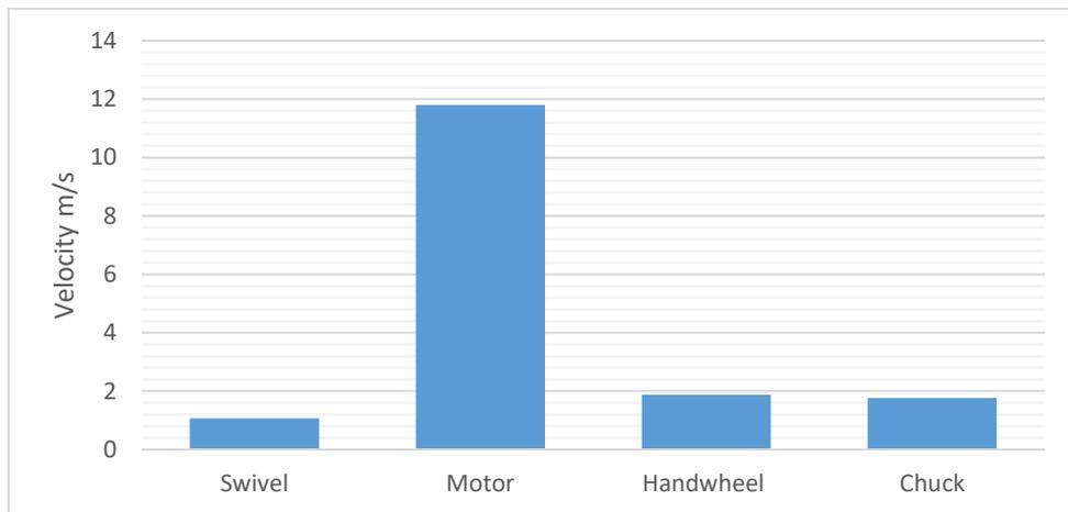
Figure 2: Measured values of velocities at different points in the drilling machine at no-load condition
