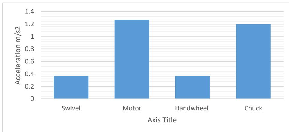
Figure 1: Measured values of acceleration at different points in the drilling machine at no-load condition
