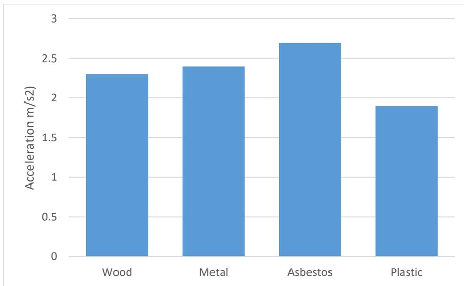
Figure 2: Measured accelerations on the electric motor for various materials
