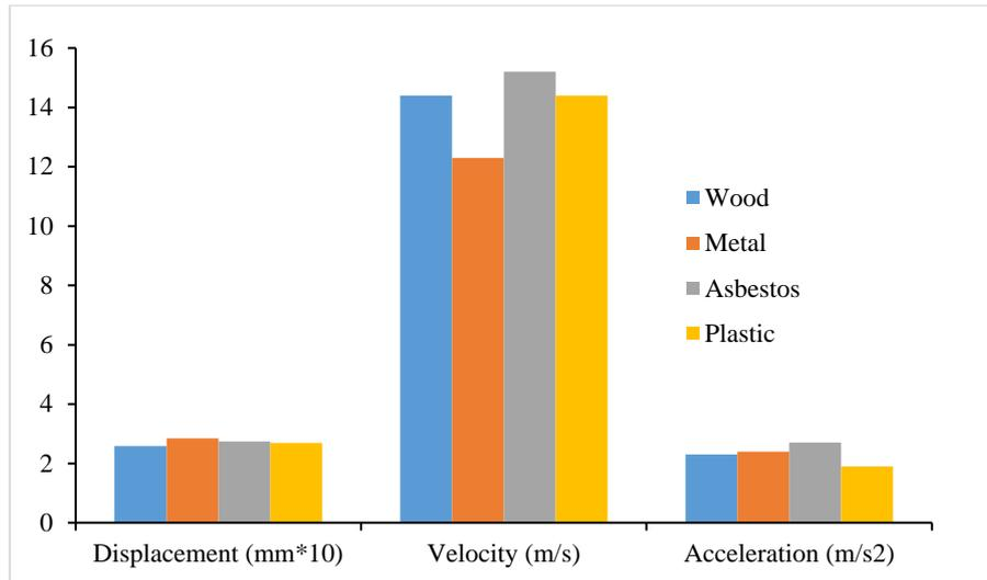
Figure 2: Measured vibrations on the electric motor for various materials
