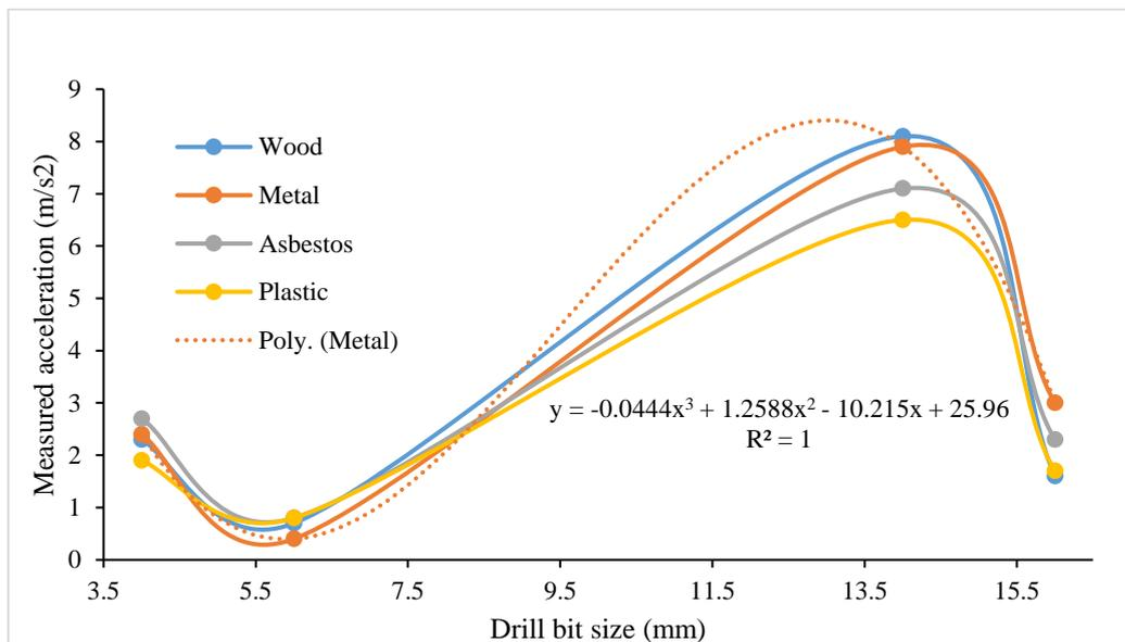
Figure 9: Values of acceleration obtained for varied bit size
