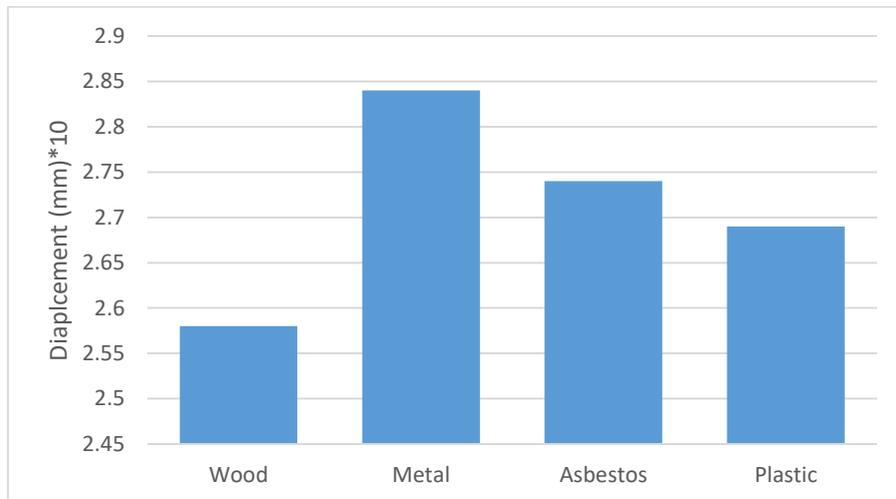
Figure 4: Measured amplitudes on the electric motor for various materials
