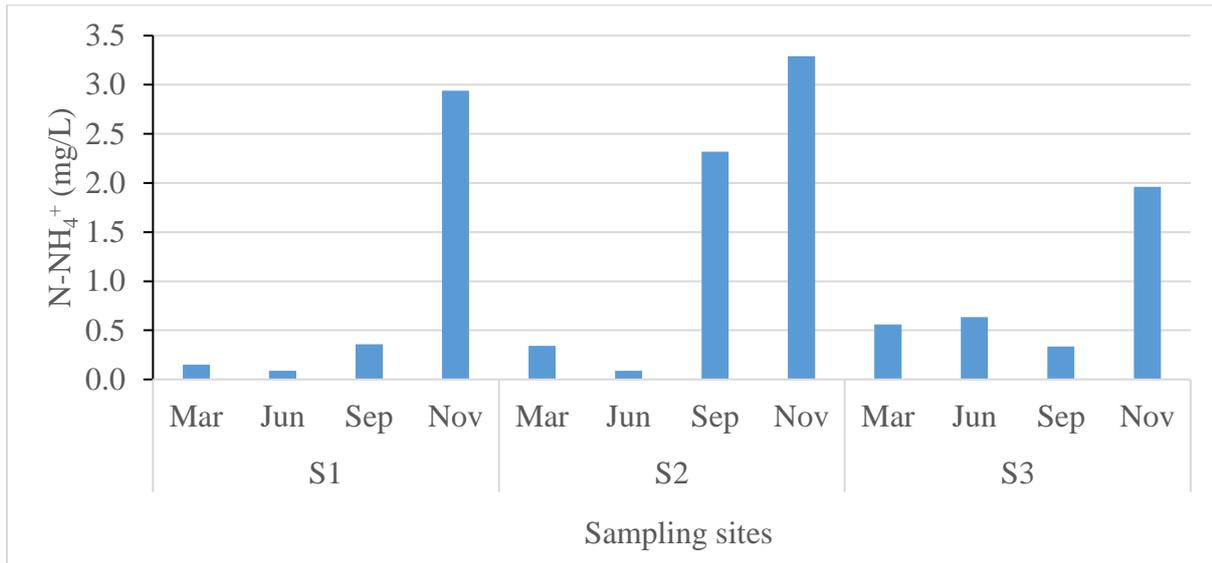
**Figure 6.  $N-NH_4^+$  in the water bodies influenced by industrial wastewater effluent**
