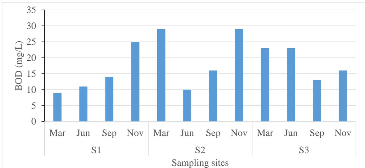
**Figure 5. BOD in the water bodies influenced by industrial wastewater effluent**
