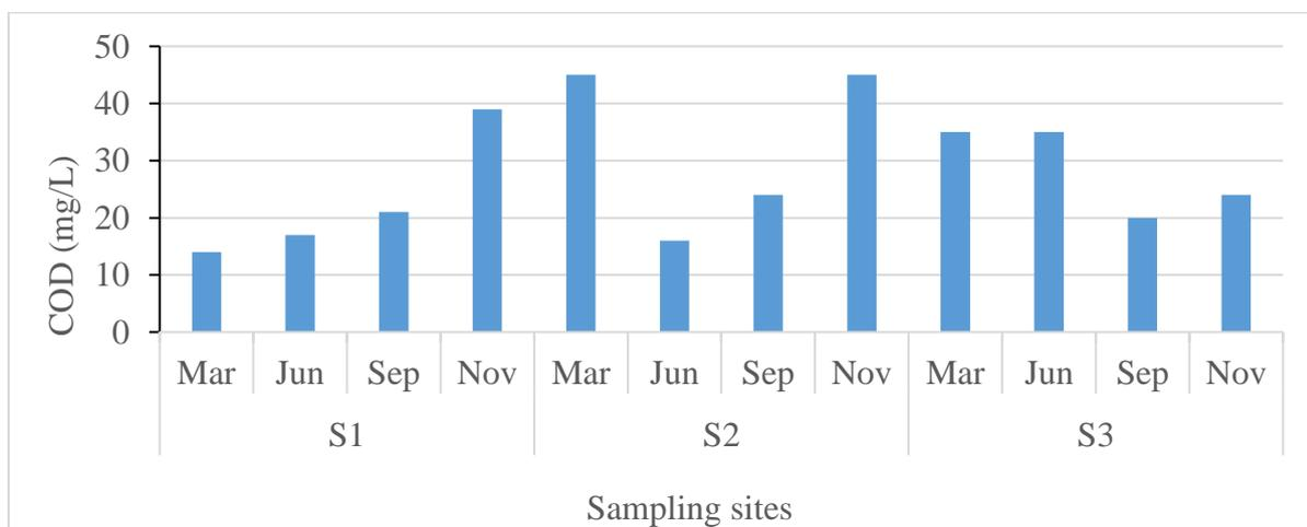
**Figure 4. COD in the water bodies influenced by industrial wastewater effluent**
