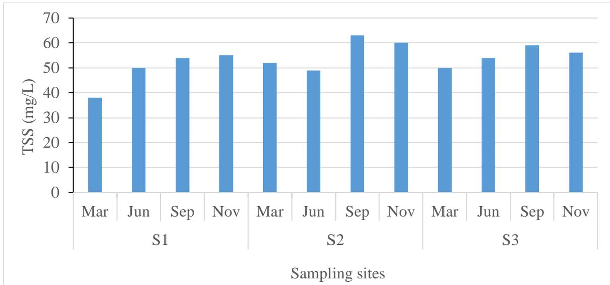
**Figure 3. TSS in the water bodies influenced by industrial wastewater effluent**
