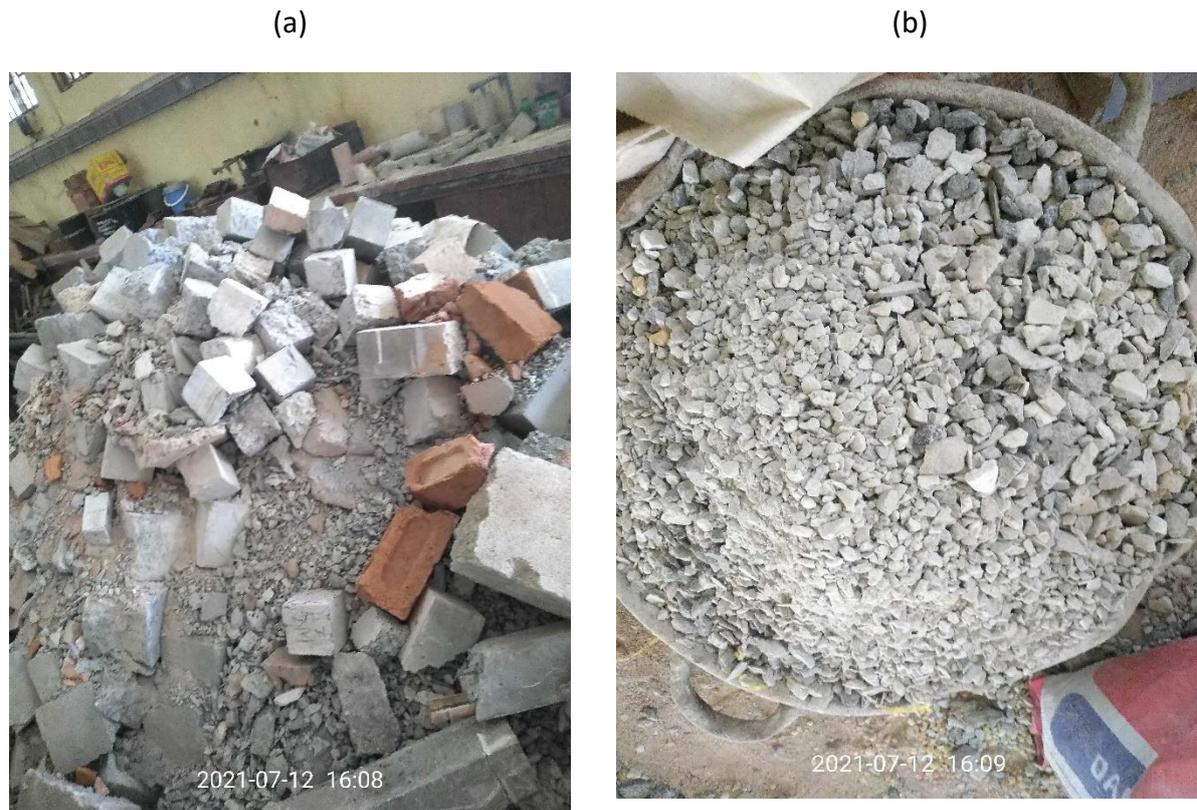
Plate 1: (a) Recycled concrete dumpsite (b) Extracted aggregates from the recycled concrete
