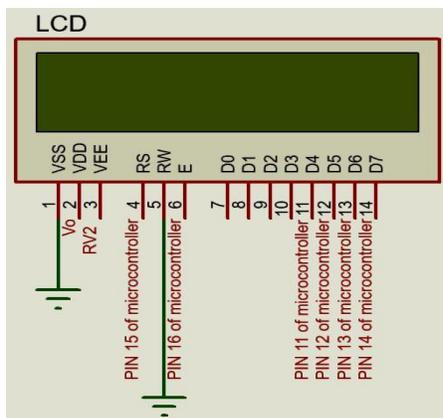
Figure 7 Circuit diagram of an LCD.
