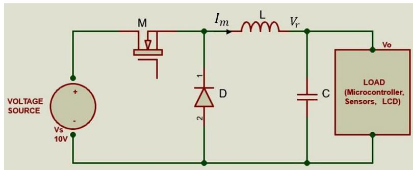
Figure 3 Buck Converter Circuit
