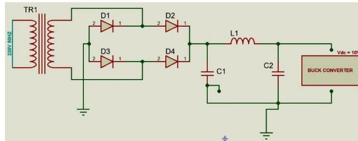
Figure 2 Circuit diagram of the Power Supply Unit
