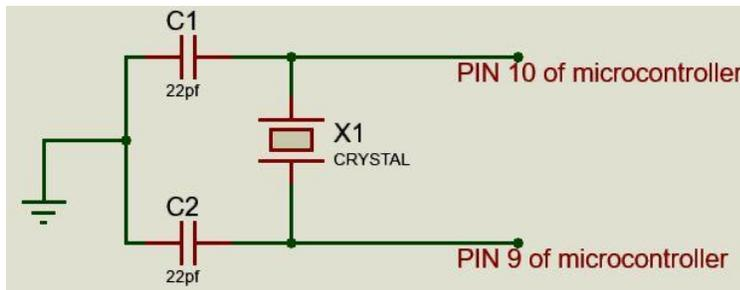
Figure 4 Circuit diagram of a Crystal Oscillator
