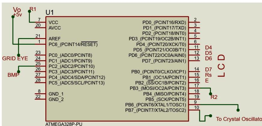
Figure 5 Microcontroller Pinout
