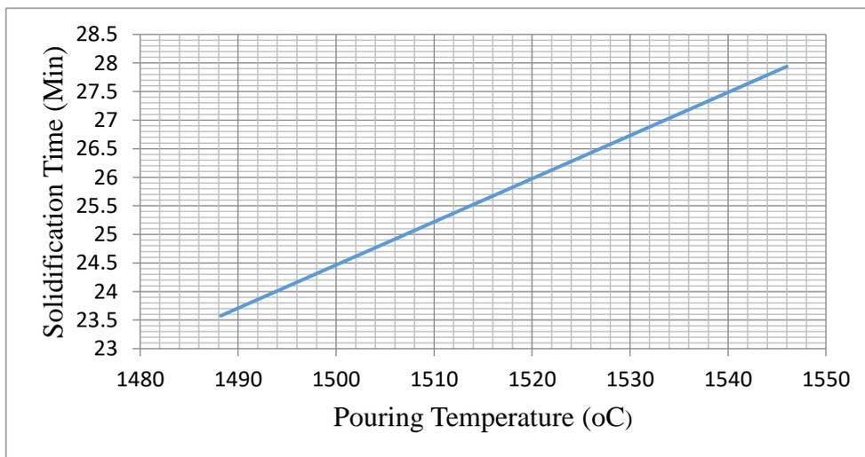
**Figure 3: A graph of Solidification time against Pouring Temperature**
