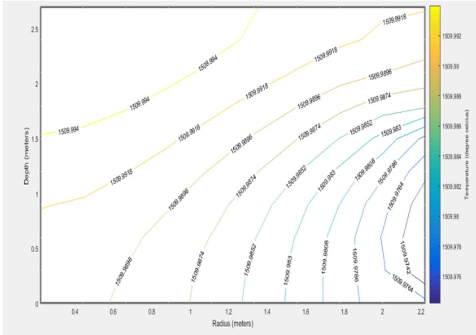
**Figure 4: Prediction of temperature distribution of the molten metal in zone 2**
