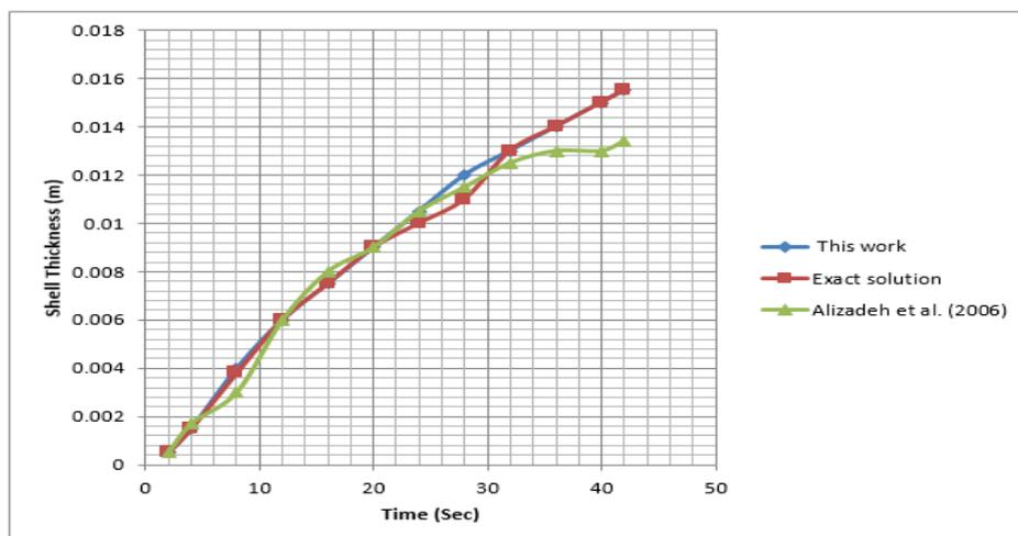
**Figure 7: A graph showing result from this work, Exact Differential Equation Method and [4] in the metal cast region**
