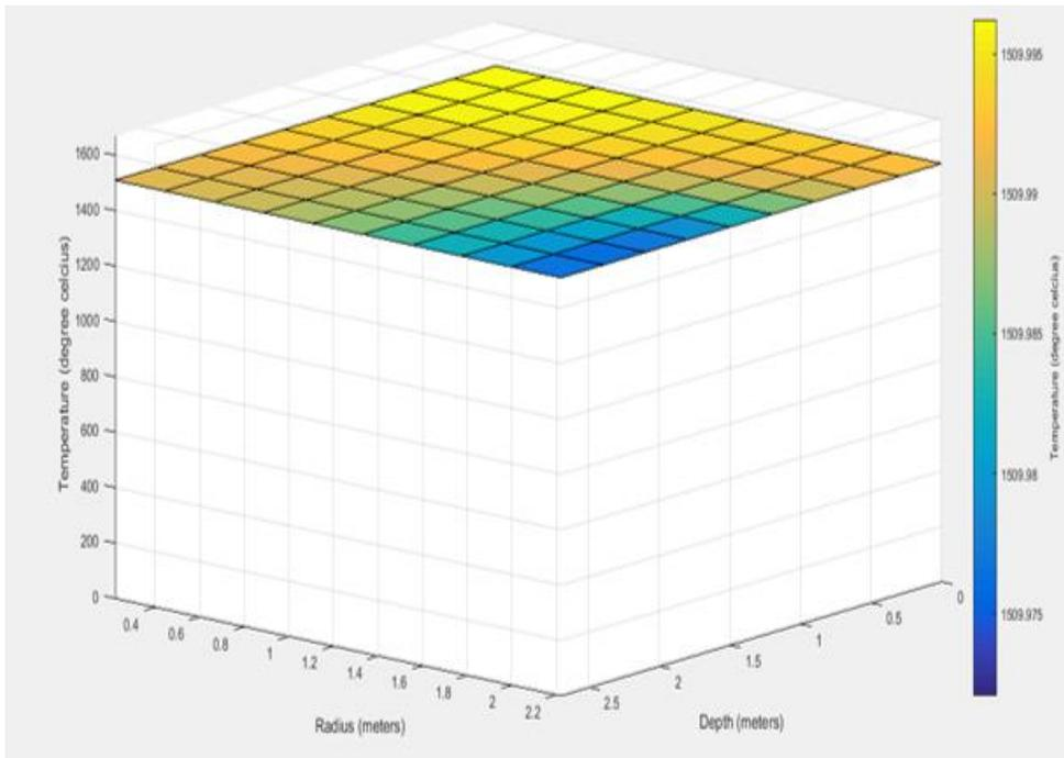
**Figure 5: Temperature distribution of the cast metal in zone 2 using surface plot**
