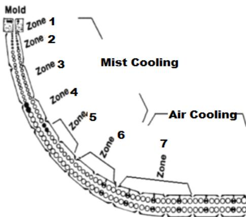
**Figure 1: Secondary cooling of the various zones**
