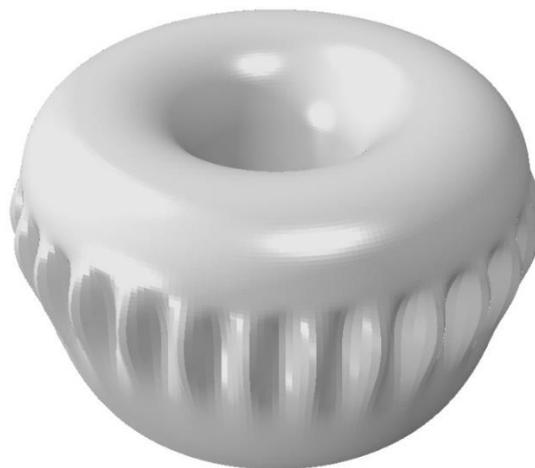
Figure 2 (b): S4R first buckling mode for a toroid with  $b/a = 3.0$ ,  $A/a = 2.0$ ,  $a/t = 200$ ,  $n = 27$
